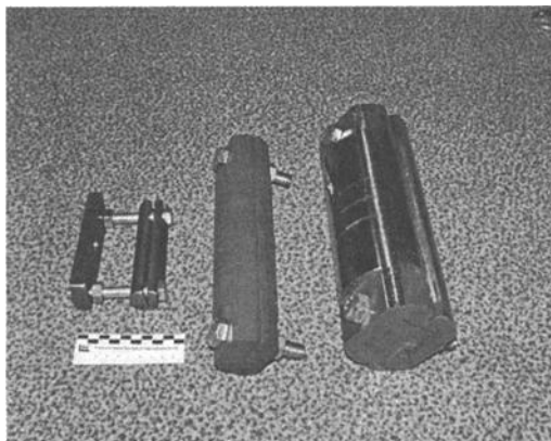
Figure 13 – capstan clamps of different roller diameters
