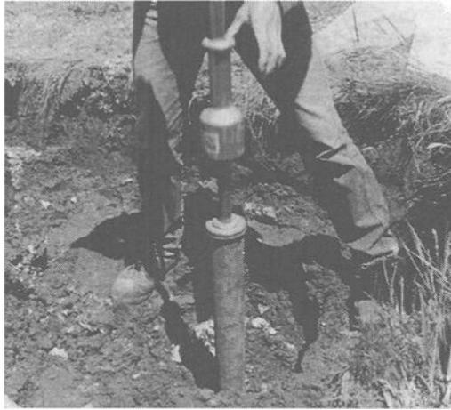
FIG. 6 -- Sampling combined sludge in tubes using 4.5 kg drop hammer.
