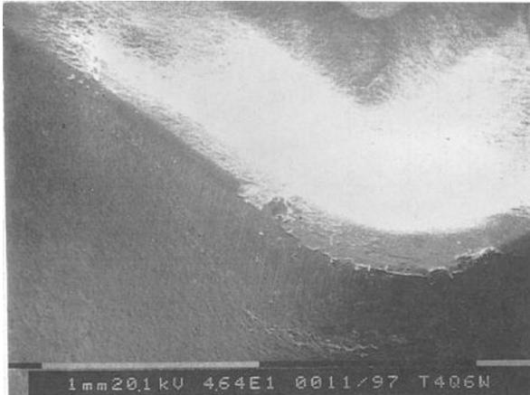
FIG. 3-- Excessive nose wear and plastic deformation on T2 at high cutting speeds and feed rate.
