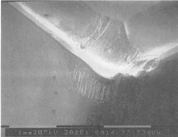
FIG. 4-- Excessive nose wear and chipping/fracture on T1 at high cutting speeds.
