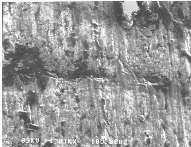
FIG 15 -- *Wear of flank face, X1000 magnification, thermal pitting. Cutting speed 240 m/min, feed rate 0.200 mm/tooth, with coolant. The dark areas are pits.*
