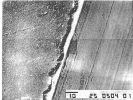
FIG. 5--Slitting edge of a top blade with completely flaked off DLC coating after use.
