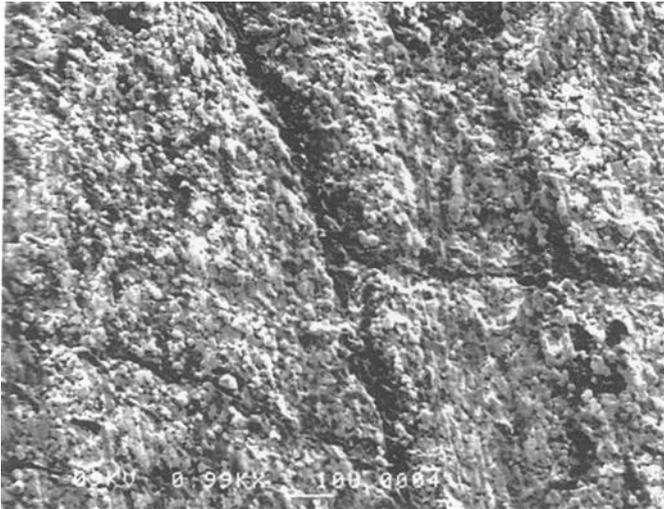
FIG 9 -- Wear of flank face, X1000 magnification. Cutting speed 360 m/min, feed rate 0.125 mm/tooth, dry cutting. Thermal fatigue cracks are perpendicular or normal to the cutting edge.
