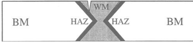
FIG. 1—Two constraints in a weldment: geometry constraint caused by crack size, specimen dimension and loading mode, and material mismatch constraint due to inhomogeneous material plastic properties.
