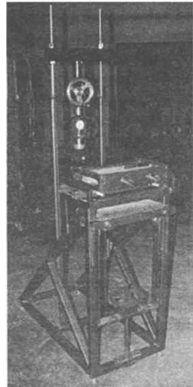
Figure 1 - Standard bond wrench testing apparatus
