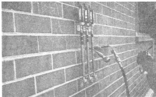
Figure 6 - Gauge Setup on Prism
