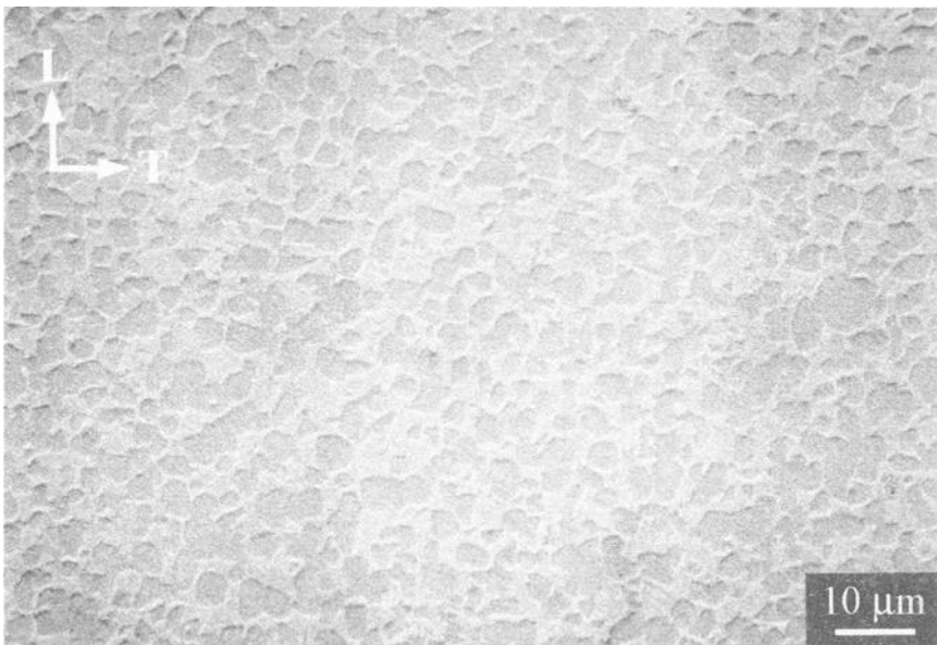
FIG. 1—SEM micrograph of Ti-62222 microstructure.
