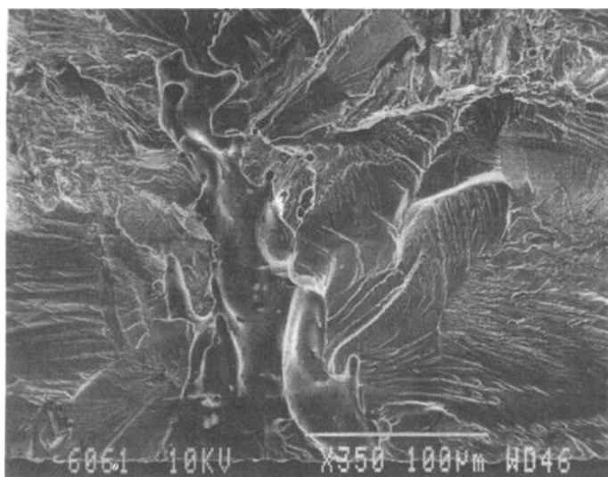
(b) Lot No. 224251, Specimen No. FS2-2, fatigue life of 109,227 cycles
