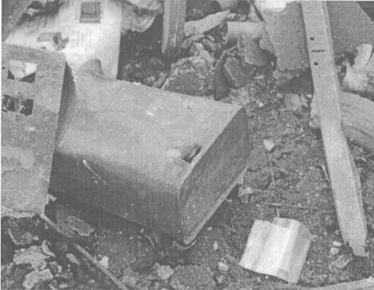
FIG. 3--Punctured fuel containers recovered in fire debris.
