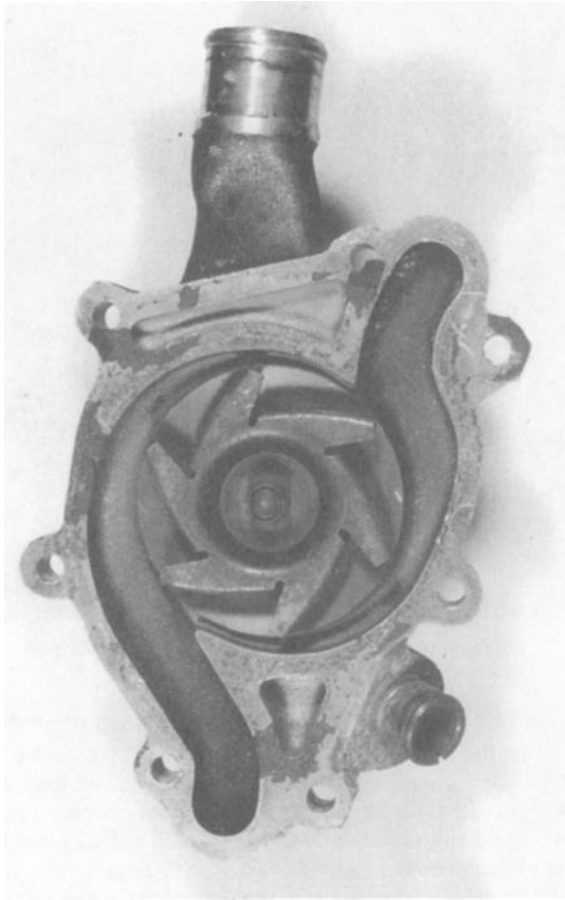
FIG. 14—Aluminum water pump protected by silicate coolant.
