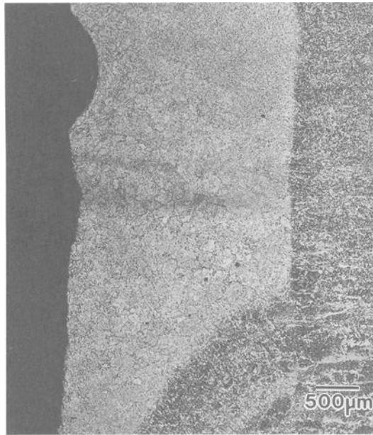
FIG. 10--Light micrograph of the initiation microstructure. 5% Nital etch
