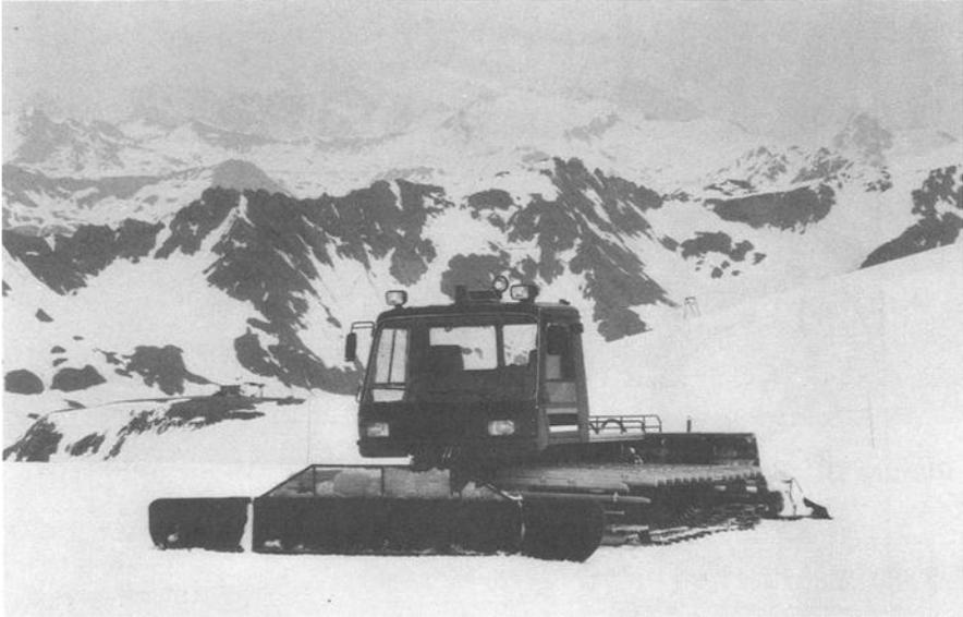
The propel drive of this vehicle consists of a diesel engine and a splitter box which drive two series 20 variable displacement axial piston pumps (Pictures 2 + 3). Each pump powers a series 20 fixed displacement axial piston motor which, through planetary gearboxes, drives the tracks. The maximum pump speed and pressures are 2800 rpm and 420 bar (6000 psi) with average pressures of 250 to 300 bar (3600 - 4300 psi).
