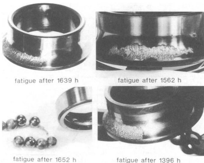
**Figure 5** Bevel ball bearing assembly run using an HFC hydraulic fluid in an axial-piston pump.
