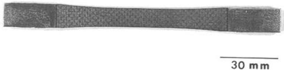
Fig. 1. SiC/SiC composite tensile specimen used in this study.
