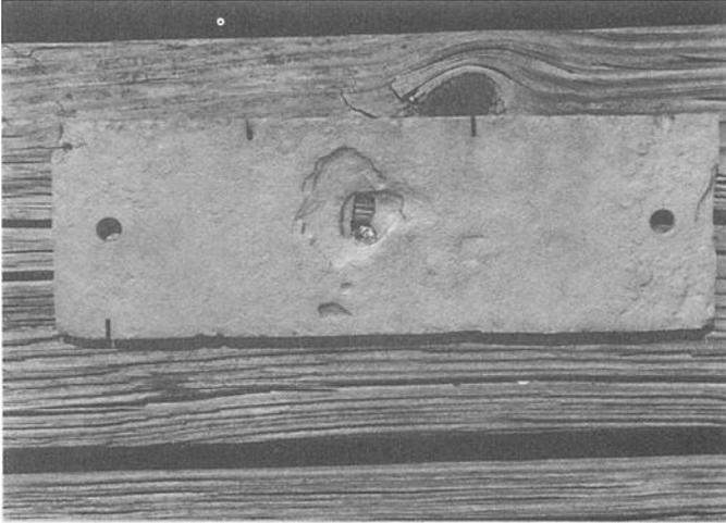
FIG. 13--Steel perforated after 1 year of exposure at the Hawaii test site. The specimen was mounted horizontally.
