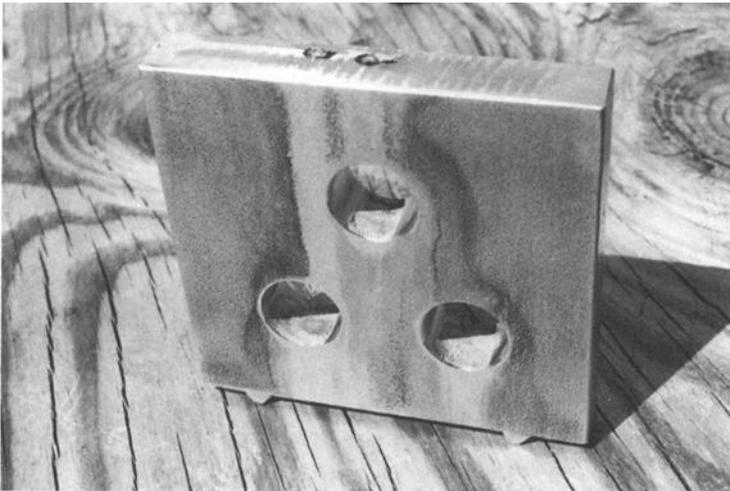
FIG. 7--Crevice corrosion at S30400 center support plate sites.
