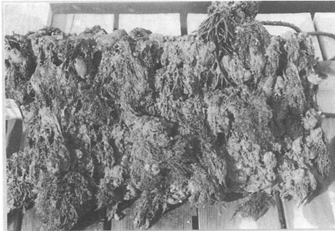
FIG. 10--Typical biofouling on carbon steel specimens after 3 years' exposure at Wrightsville Beach, North Carolina.
