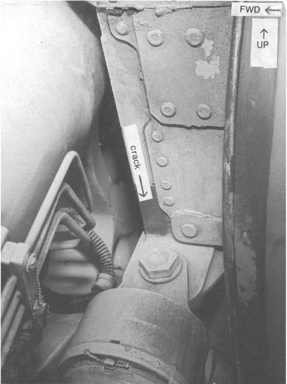
FIG. 3—*Photograph showing main landing gear trunnion lug and retract cylinder attachment lug.*
