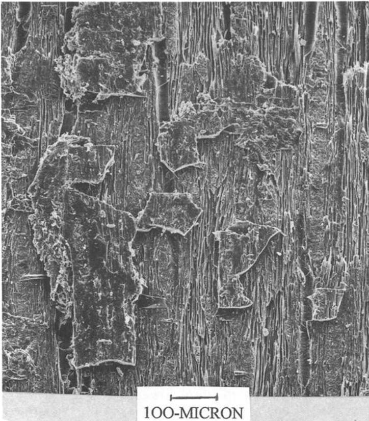
FIG. 10—Sanded (abrasive planed) surface of Maple before laminating into bowling pin (compare to Fig. 2, also maple).
