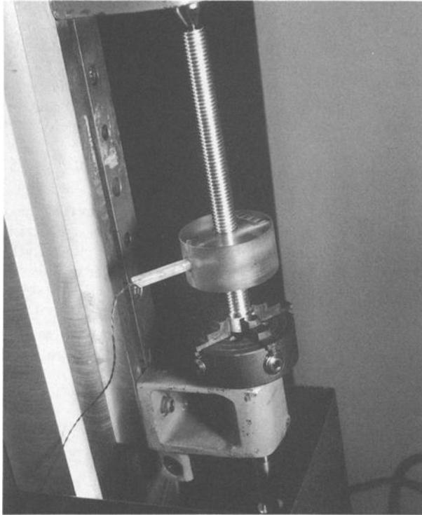
FIG. 6—Close-up photograph of eddy current inspection of threaded aluminum rod.
