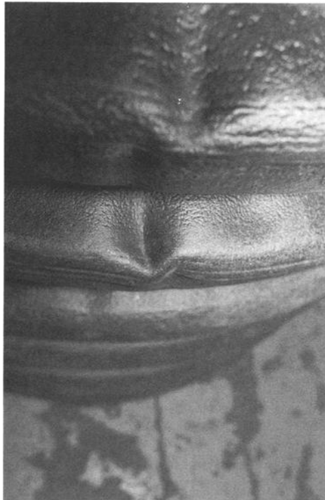
Fig. 11 Local Buckling of Corrugation Wall
