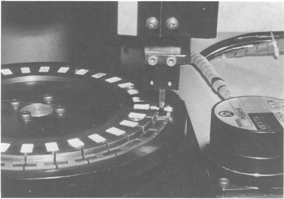
FIG. 8—Specimen arrangement in specimen tray. The turntable rotates until a slit of an entered number comes into position and a specimen is inserted into the slit.
