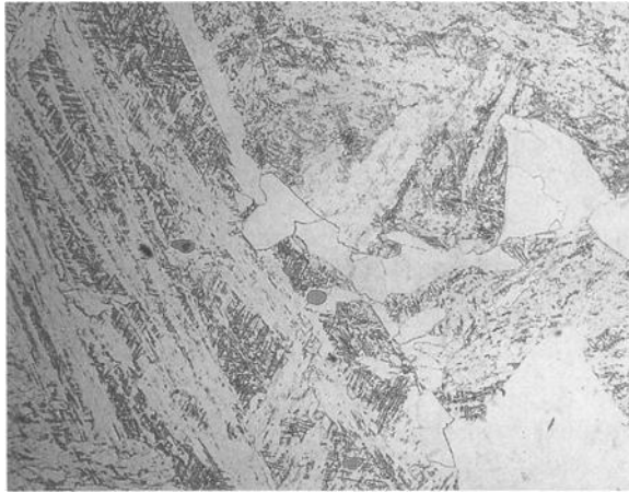
FIG. 3—Microstructure showing lath martensite structure ( \times 400 ).
