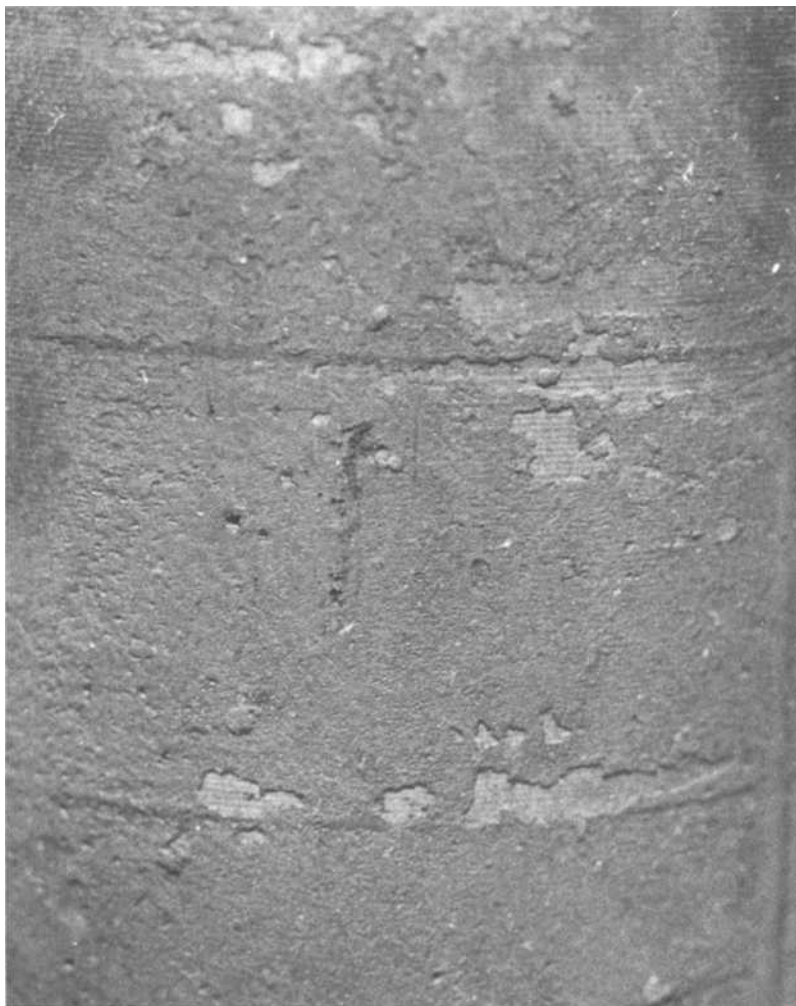
FIG. 16—Coolant side of a cylinder liner fouled with oil sludge.
