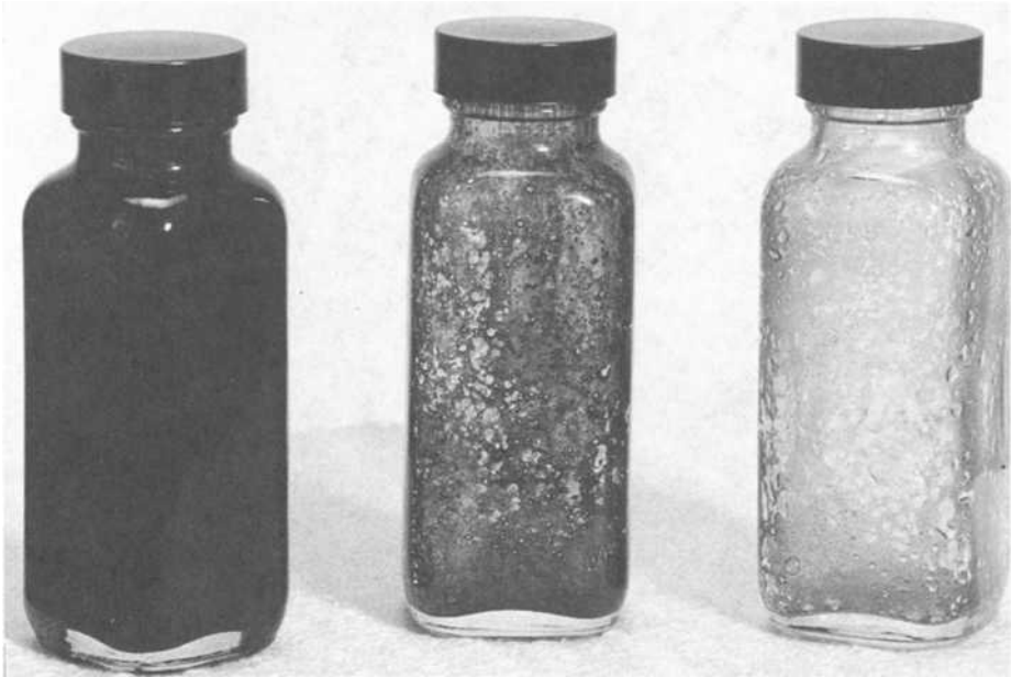
FIG. 18—Detergency test of SCAs. First bottle shows oil coating sides before testing. Middle bottle is results obtained from a borate-nitrite SCA while bottle to the right was obtained with the phosphate-molybdate SCA.
