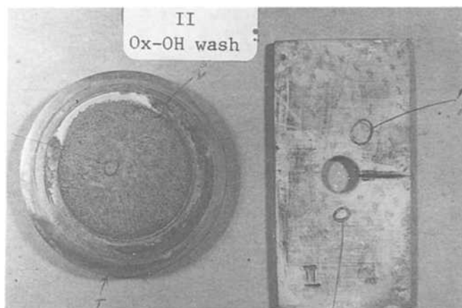
FIG. 5—The heat-rejecting iron disk and heat-accepting iron coupon after cleaning with oxalic acid.
