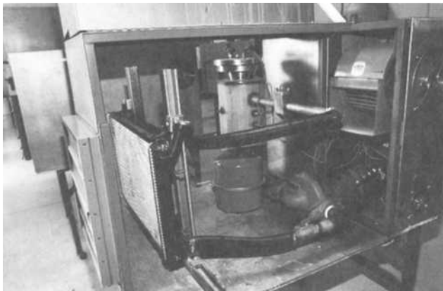
FIG. 12— Installation of radiators in radiator test frame.
