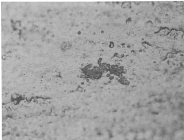
FIG. 24—Shallow pit in unclad tube after 8 weeks in Oyama water.
