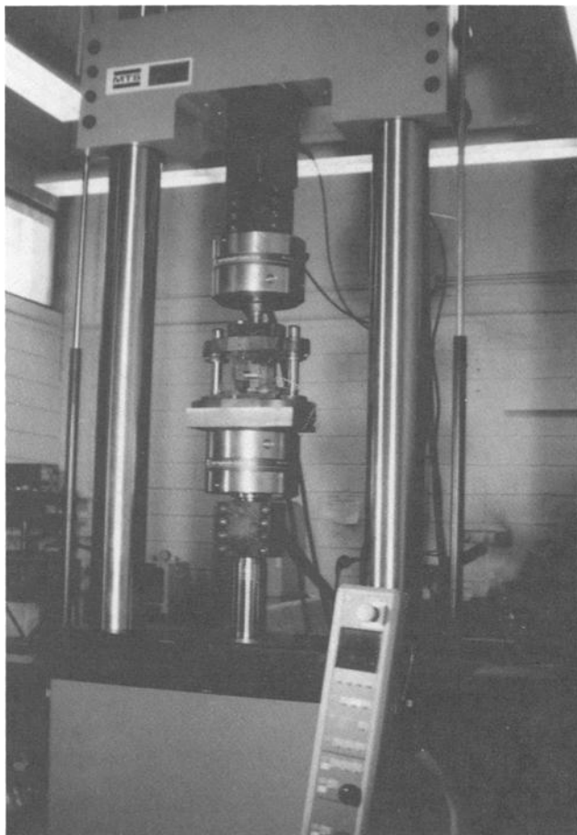
FIG. 8— Photograph of anticlastic bending loading apparatus in a fatigue testing machine.
