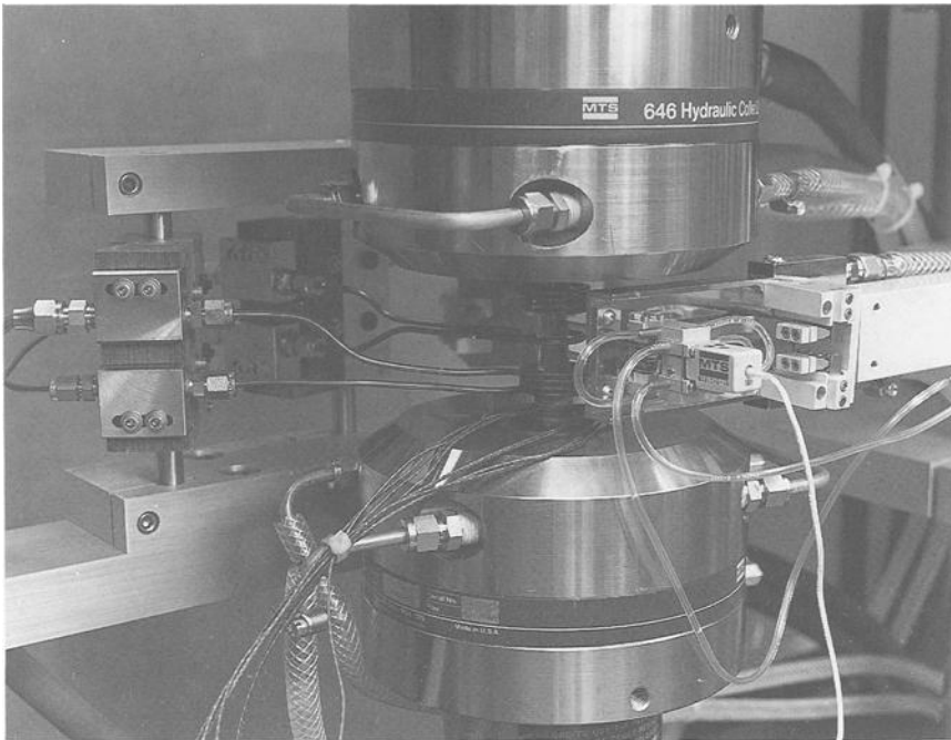
FIG. 4— Experimental setup used for thermomechanical testing.
