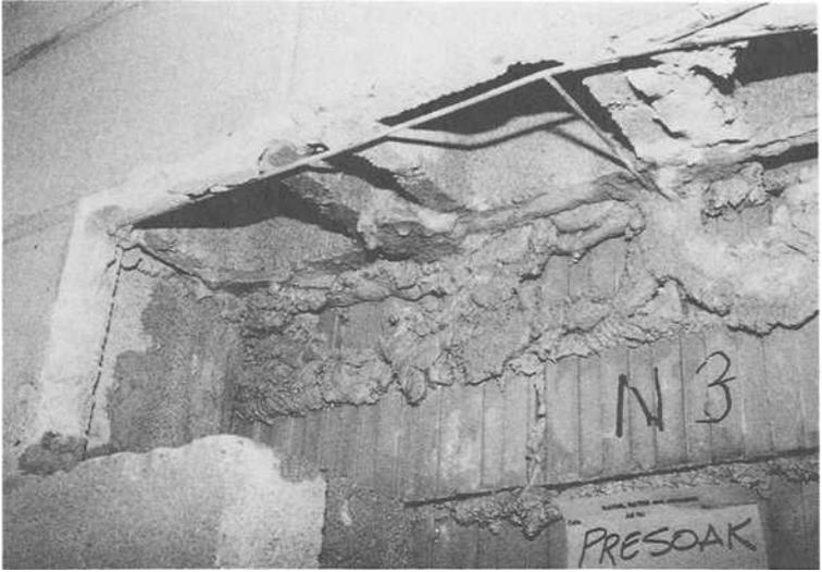
FIG. 4 -- Water from test presoak has bridged cavity and is dripping through cores of CMU back-up.
