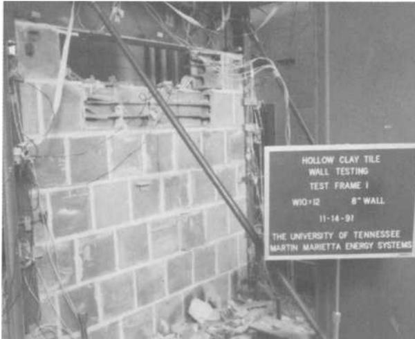
FIG. 8--Ultimate Failure Mode of Racking Tests
