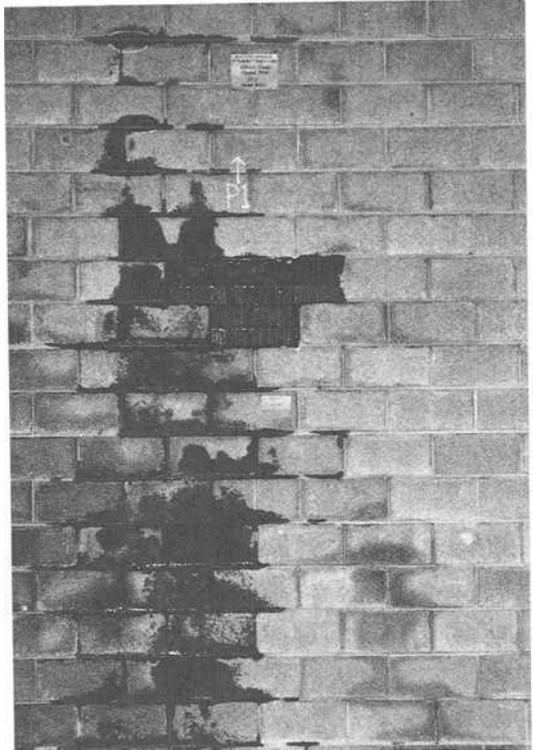
FIG. 3 -- Interior side of CMU back-up is saturated during field E 514 test due to water bridging cavity space.
