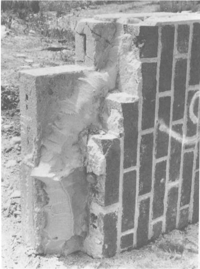
Fig. 3 -- Portion of test panel. Note dense surface of foam in contact with masonry surfaces.
