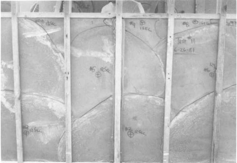
Fig. 2 -- Fully foamed test panel
