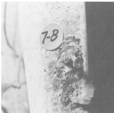
FIG. 3 - Representative bugle-head screw after 2409 hours of exposure.
