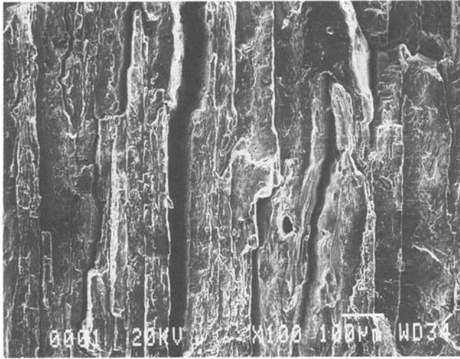
FIG. 5—Fracture surface of C(T) specimen from Alloy 2090-T81-1/2 tested at 4 K.
