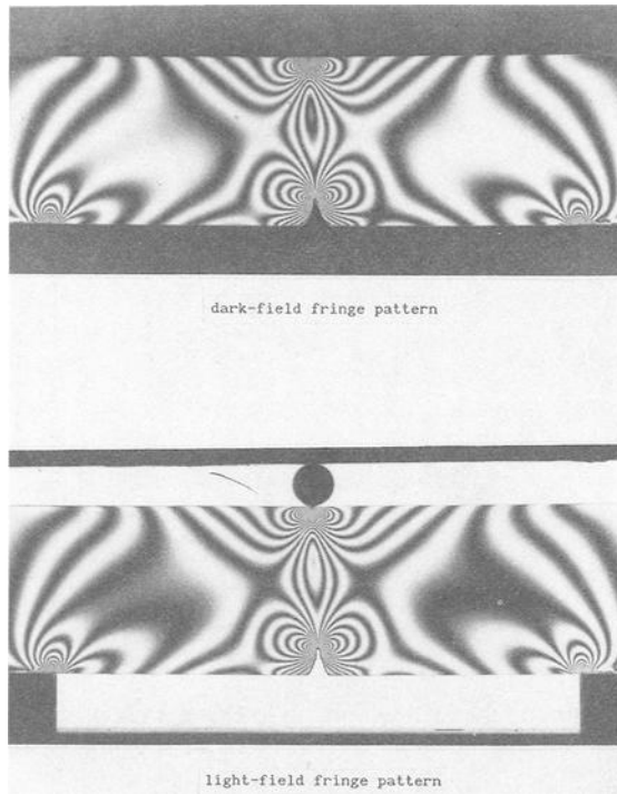
FIG. 4—Isochromatic fringe patterns for the photoelastic model.
