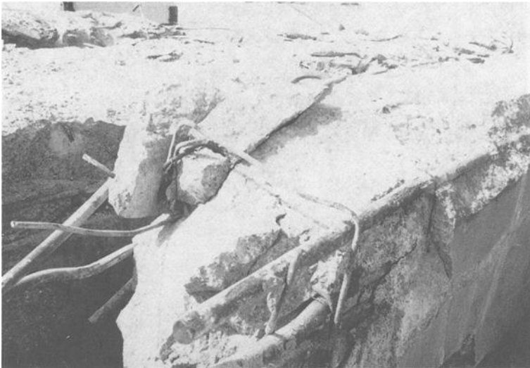
Figure 4 Pre-cast beam removed after 15 years exposure showing clean, passivated rebar in top portion of beam (left hand side of photograph).
