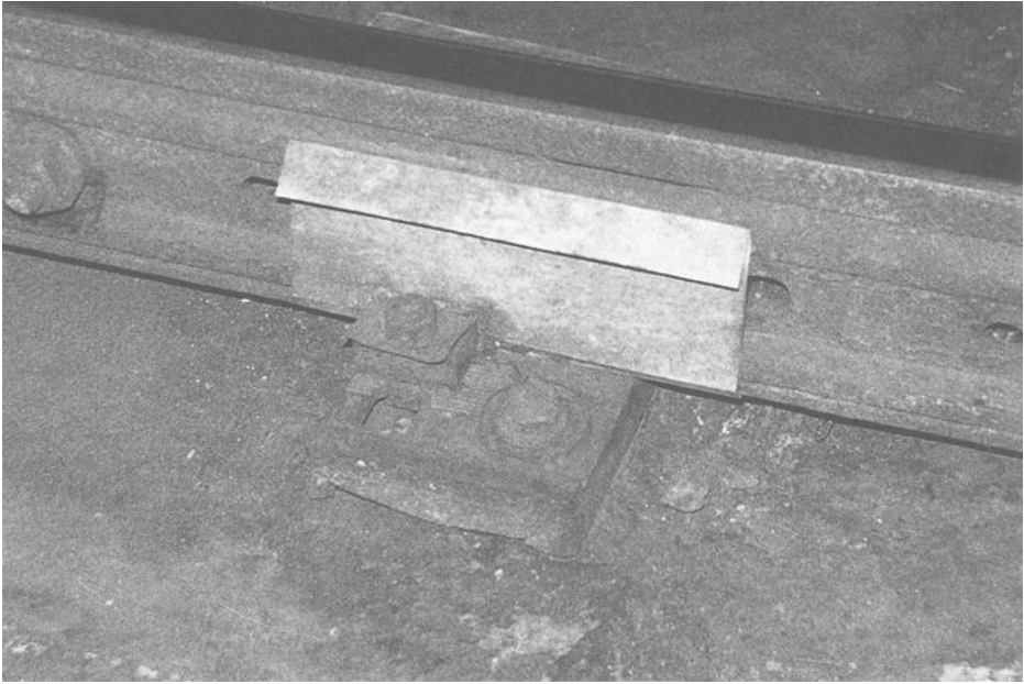
Figure 7. Photograph of Plastic Insulator on the BART System where Cracking was Common.
