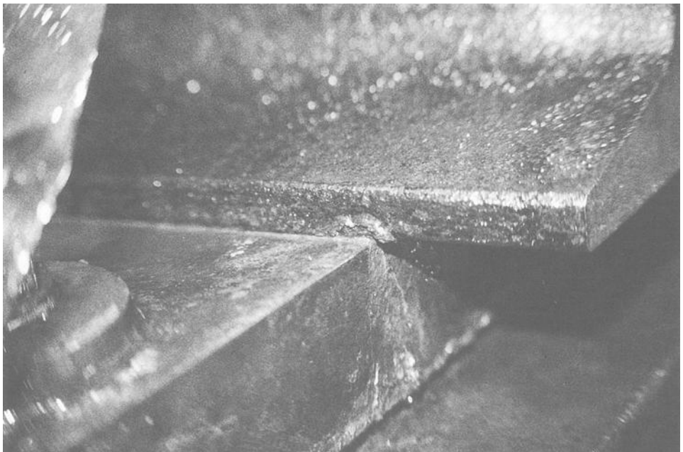
Figure 5. Photograph of Fastener in Test Chamber with Notch in Rail after one week of Accelerated Testing.
