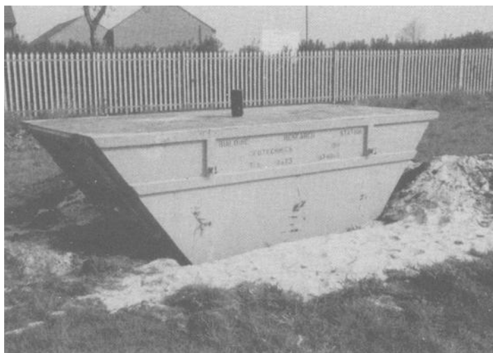
Fig. 2 In situ load test using a sand-filled skip on precast footing
