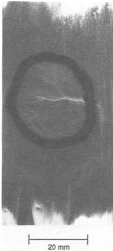
FIGURE 3 -- Surface damage indications. (S/N0785, 16.24J damage)
