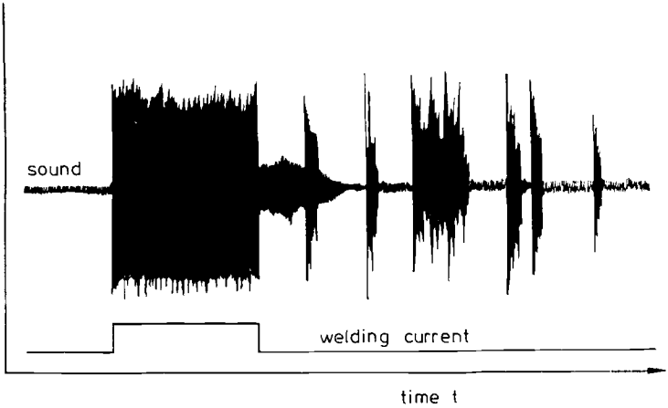
Fig. 1 : Acoustic emission from EB welding
