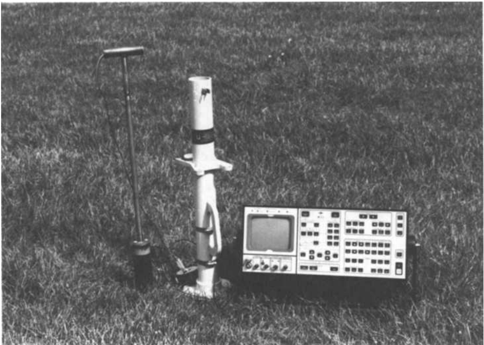
FIG. 1—Apparatus used in the assessment of impact characteristics: (left to right) impacting hammer, guide tube from Clegg impact soil tester, and Bruel and Kjaer 2515 vibration analyzer.
