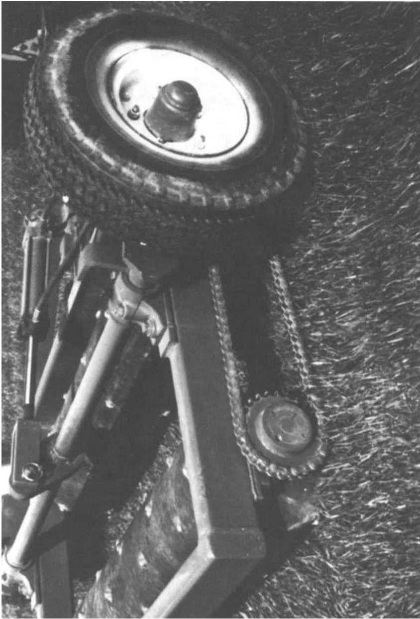
FIG. 2—The Brinkman traffic simulator chain and sprockets.
