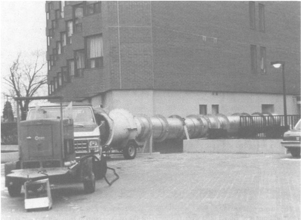
FIG. 1—Building test setup showing exhaust fan and duct connection.
