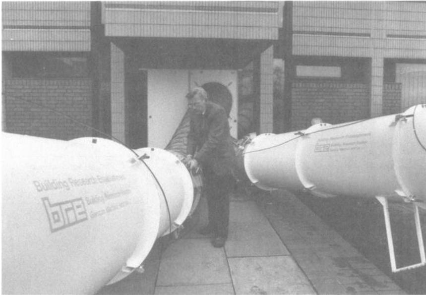
FIG. 3—Pressurization system installed in the main entrance (north face) of Building B.
