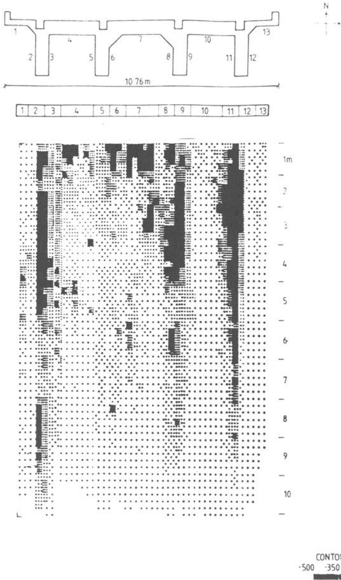
FIG. 9—Potential map of the bridge soffit.
