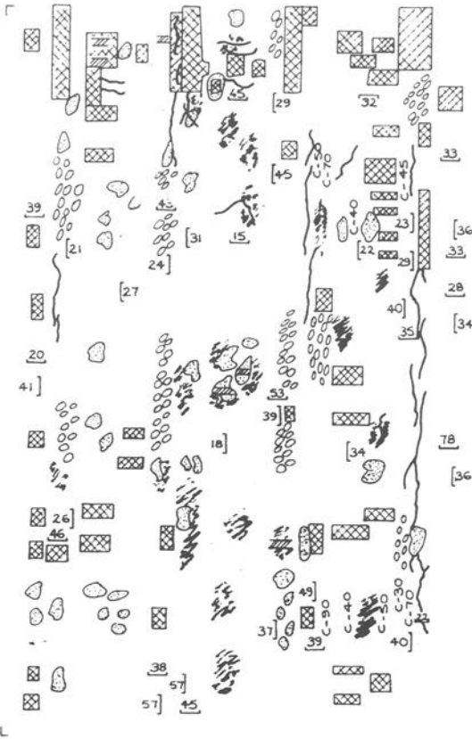
FIG. 10—Visual survey of a bridge soffit.
