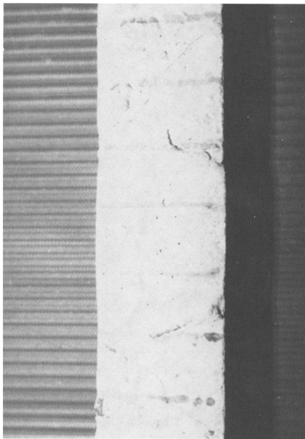
FIG. 8a—Close up view of repaired specimens after eight cycles, cracks near patch.
