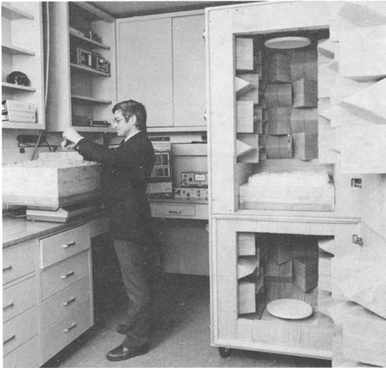
FIG. 4—Photograph of the test chamber with a sample basket installed. The operator is measuring the thickness of another sample, which is resting on a digital balance.
