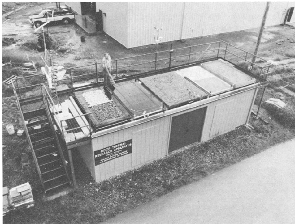
FIG. 1— Roof Thermal Research Apparatus. Roof specimens are instrumented for careful measurements and tested under field conditions.
