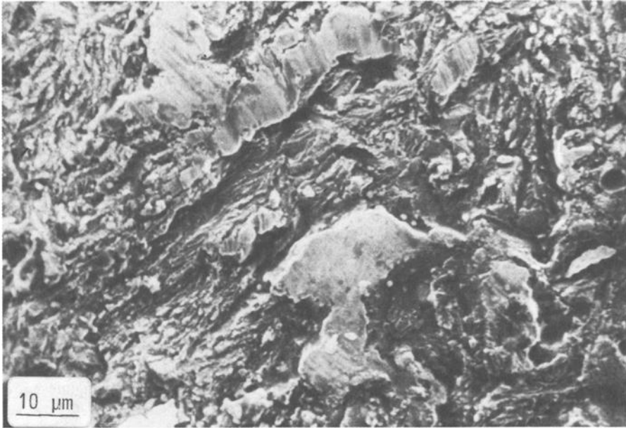
FIG. 10—Fracture surface after Mode I fatigue cracking with \Delta K_I = 6.2 \text{ MPa}\sqrt{\text{m}} , K_{II} = 12 \text{ MPa}\sqrt{\text{m}} , and R = +0.25 .
