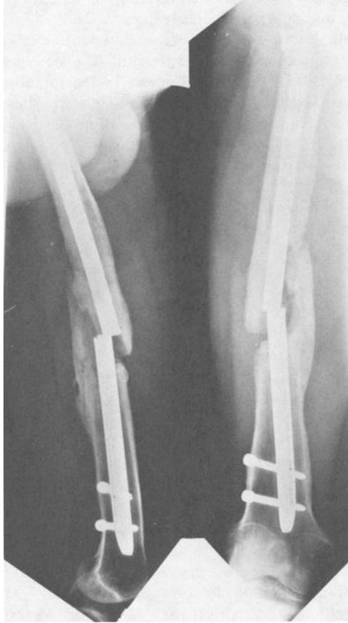
FIG. 1—Breakage of a statically locked Grosse-Kempf femoral nail 14 months following injury. The fracture has failed to unite.
