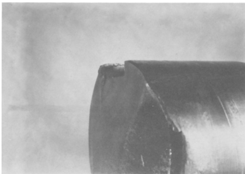
FIG. 15—Stress corrosion cracking in a second 17-4PH stainless shaft, this taken from a steel mill descaling operation. Note the crack in the keyway, parallel to the outer surface.
