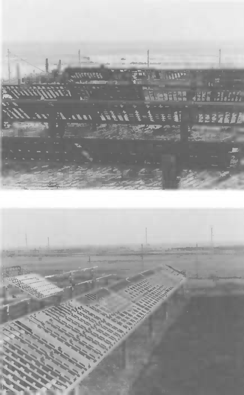
FIG. 3—Views of the atmospheric lots at Kure Beach, NC, where various grades of stainless steel have been exposed for 26 years (1958 to 1984). Top: view of 25-m lot panels facing east. Bottom: view of 250-m lot panels facing south.
