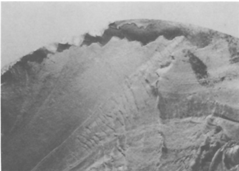
FIG. 14— Stress corrosion crack propagates from spalled region. Fatigue cracks initiate on spalled surface, some distance from keyway.
