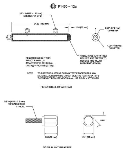
FIG. 8 Steel Impact Ram Assembly
