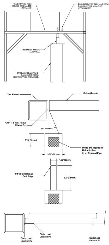
ASTM F2697 security grades and load requirements.
