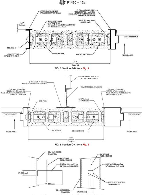
FIG. 7 Wall Anchor Welding Detention Hollow Metal Vision Systems
