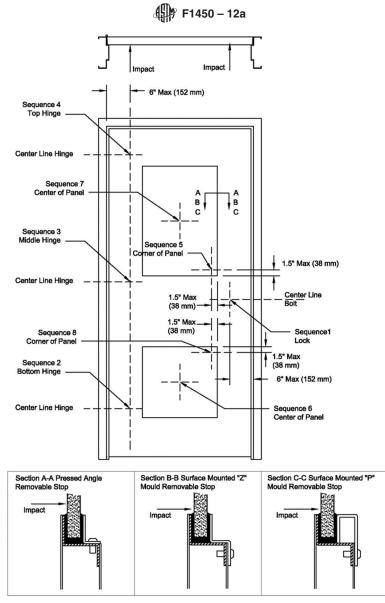
FIG. 2 Test Assembly Door Elevation #2 Location of Strike Points Described in Table 2
