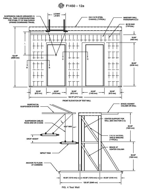
(two large vision lights), deliver the series of impacts in Table 2 (and shown in Fig. 2) to the push side of the door.
