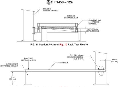
FIG. 12 Section B-B from Fig. 10 Rack Test Fixture
