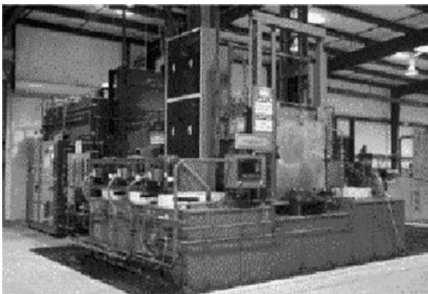
Fig. 14 —Atmosphere furnace equipped with 41-m 3 IQ water tank.
