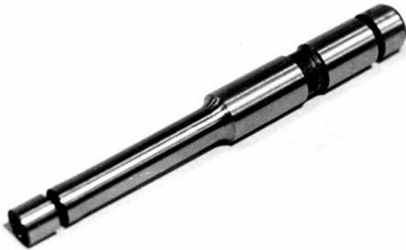
Fig. 7—Punch made of the molybdenum high-speed steel R6M5 (AISI M2). Intensive quenching in aqueous chloride solutions increased the tool life by 2.5 times. The punch is 126 mm long, and its maximum diameter is 15.3 mm. Its microstructure is shown in Fig. 8.
