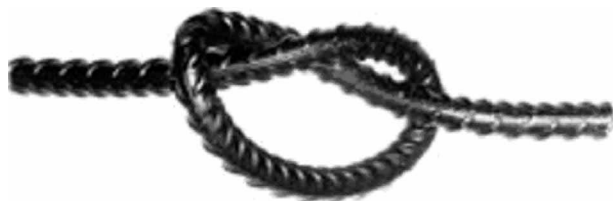
Fig. 28 —High plastic and bending properties of rebars are achieved by combining thermomechanical treatment with the intensive quenching [65].
