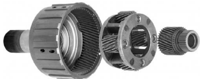
Figure 15.4—Expanded view of planetary gear set.
