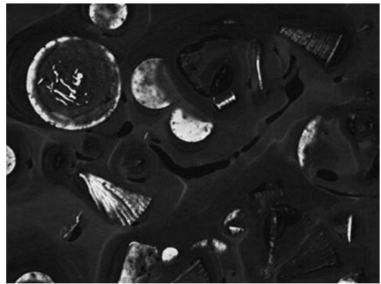
Figure 21.31 —Oxidation converts the low-viscosity oil to a mass resembling asphalt.
