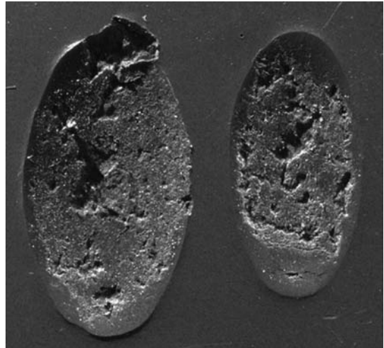
Figure 21.18 —Melt wear on polyimide (PI) surface.
