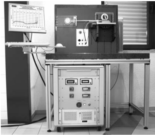
Figure 21.47—Oscillating friction tribometer.
