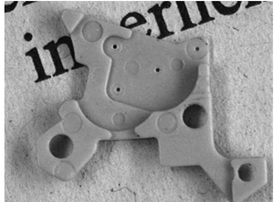
Figure 21.2 —Bearing in a housing made of poly(butylene terephthalate) (PBT). Diameter 0,2 mm.
