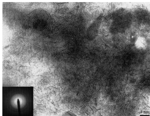
Figure 20.46 —The TEM of wear debris showing the presence of MoS 2 "eyelashes" [131].
