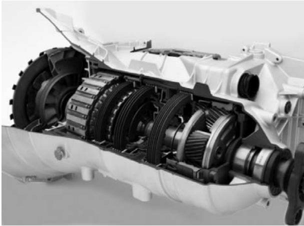
Figure 15.5 —Cutaway of an AT with a good view of the torque converter clutch, shifting clutches, and planetary gear set.
