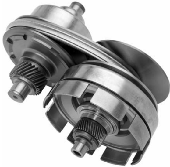
Figure 15.8 —Van Doorne push-belt CVT variator pulley and belt arrangement.
