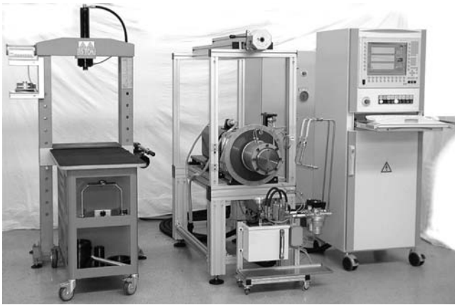
Figure 9.16 —FAG FE8 lubrication grease's life test rig. 1 = workshop press, 2 = workshop carriages, 3 = test units, 4 = control cabinets, and 5 = PC with evaluation software.
