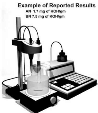
Figure 22.7 —Potentiometric titrometer used to determine ANs and BNs.
