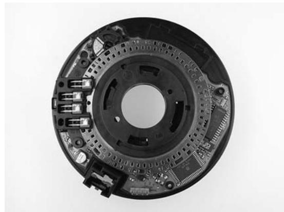
Figure 21.8—Angle of rotation generator in the steering wheel.
