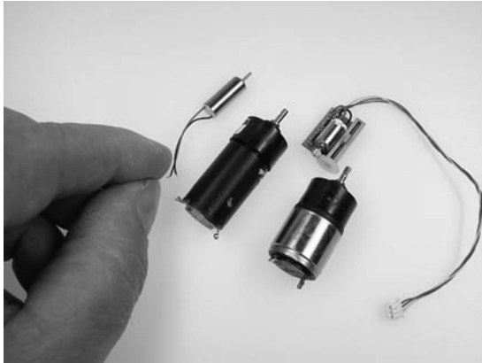
Figure 21.4—Miniature motors with planetary gears.
