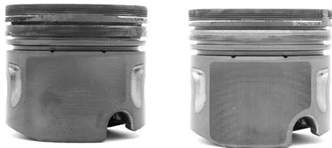
Figure 2.25—Examples of poor (left) and good (right) detergency.
