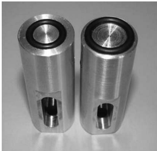
Figure 21.48—Specimen holder for different types of o-rings.
