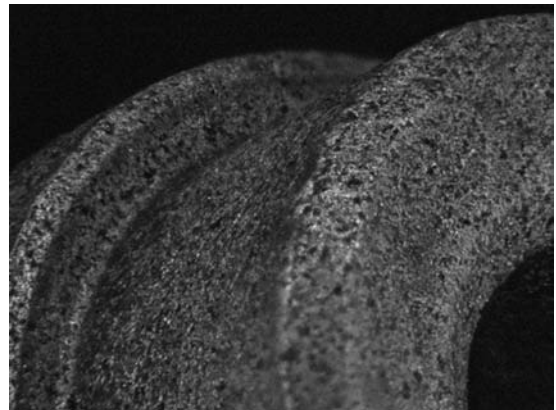
Figure 21.3 —Sintered bronze bearing, 2 mm inside diameter. The pores are clearly visible.
