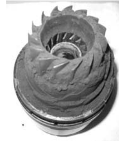
Figure 24.3 —Sectioned view of a centrifuge field return from Saudi Arabia (contained 75 % sand).
