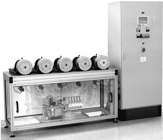
Figure 9.17 —FE9 test rig with five test units. 1 = frame, 2 = oil unit, 3 = test units (5 pieces), and 4 = control cabinet with actuator.
