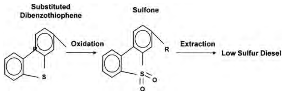
Figure 9.17—A reaction mechanism for oxidative desulfurization.
