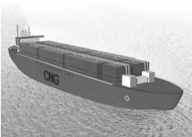
Figure 11.34 —Trans Ocean Gas CNG ship (FRP). Source: Picture courtesy of Trans Ocean Gas, Inc.
