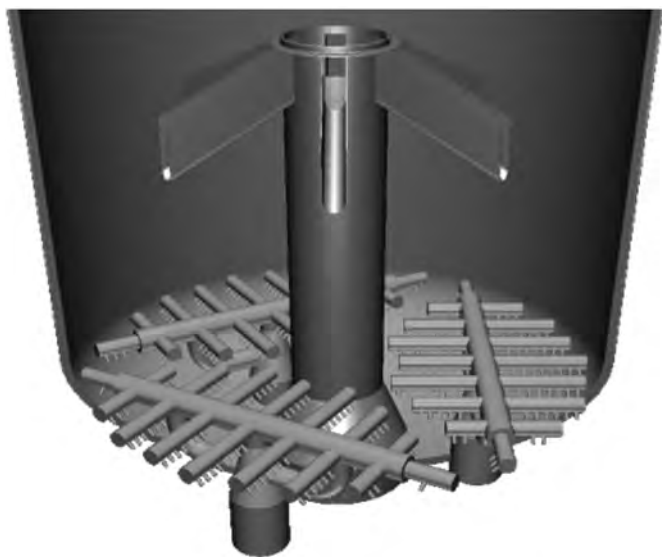
Figure 6.14 —Schematic of spent catalyst distributor and air distributors in KBR's FCC regenerator. Source: Figure used courtesy of KBR, Inc.
