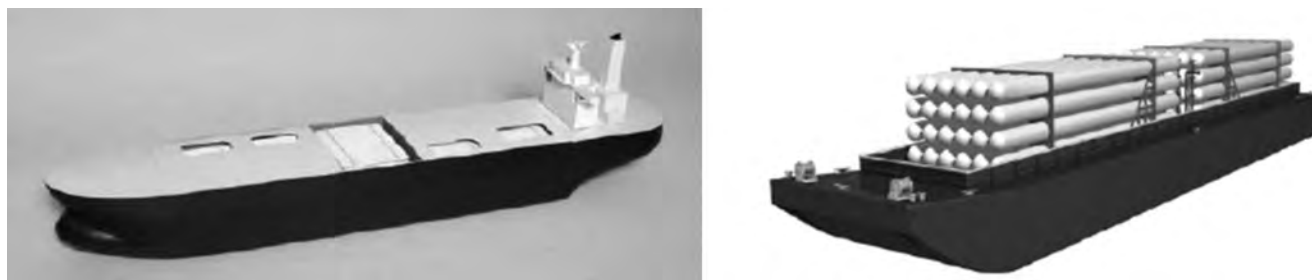
Figure 11.31—Conceptual ship and barge design using GTMs. Figure courtesy of TransCanada, all rights reserved.
