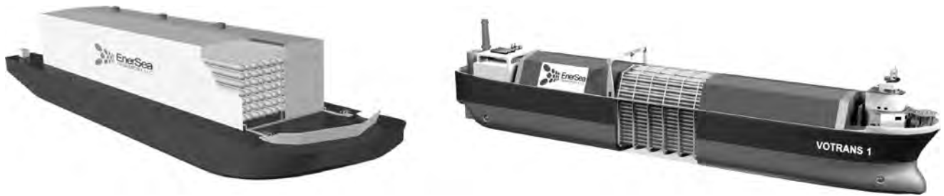
Figure 11.33 —EnerSea's CNG barge and ship (VOTRANS). CNG can be delivered using EnerSea's VOTRANS CNG marine service with ships (right) or barges (left) as shown in the illustration.
