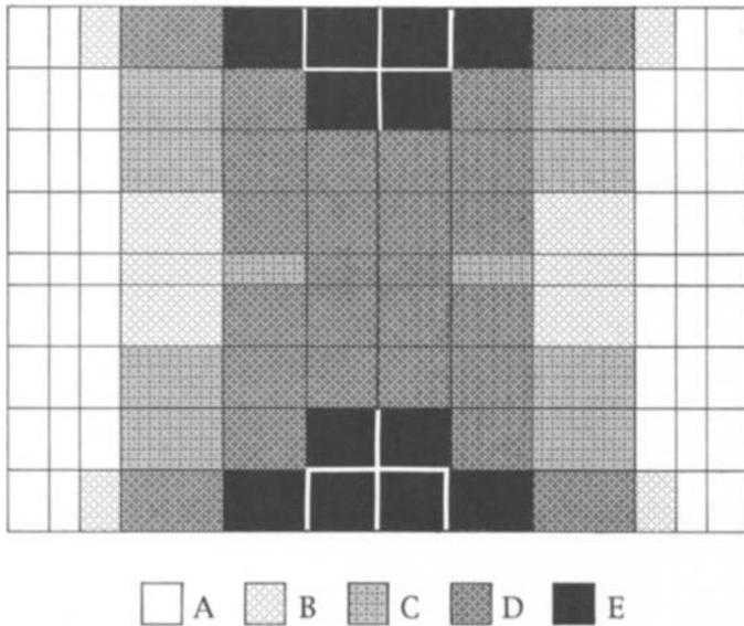
▲ FIGURE 124: *Finite Element Model Matrix.* To improve the accuracy of the theoretical mathematical model, the grid of plate bending elements was arranged to create the smallest elements where the largest stress gradients and maximums occurred, typically near supports and midspans.
