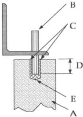
◀ FIGURE 98: *Dowel Anchor Mechanics.* Dowel engagement is the length of anchor (B) embedded (D) in the stone (A). Maximize embedment of the anchor into the drilled hole (E) without bottoming the dowel. Fill the hole with compressible material (typically sealant) that cushions the anchor and distributes the pressure of the support reaction along the hole's full depth. Alignment of the dowel (B) and the hole (E) is critical to preventing prying points-of-contact at the rim of the hole (C).
