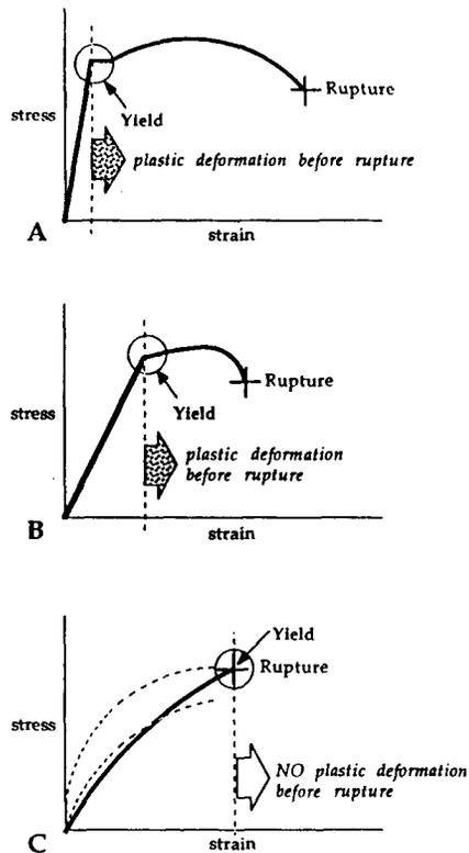
◀ FIGURE 32: *Stress-Strain Behavior Of Natural Stone Compared To Other Common Facade Structural Materials.*
