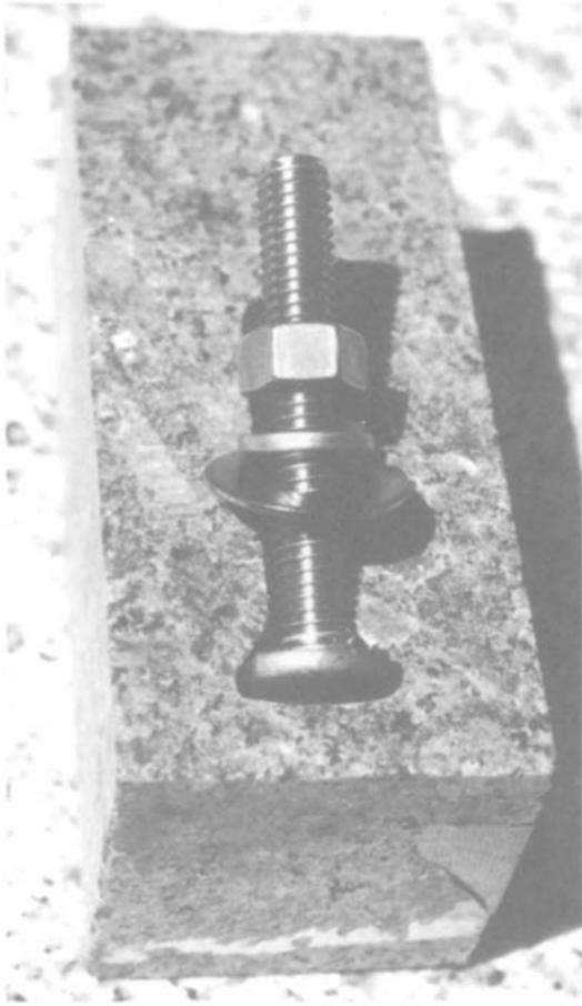
◀ **FIGURE 79: Headed Shank Anchor.** Also popular as a “type #31” patented by Cold Spring Granite Company, this effective device uses the advantages of an eisenshank’s large potential failure cone and an inclined rod-and-plug’s placement anywhere in the stone. A special diamond bit routes a slot into the stone, and an
