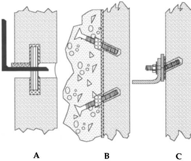
◀ **FIGURE 68: Anchor Types That Fit Into Single Drilled Holes.** Devices that engage a single drilled hole in the stone include a dowel typically in the top and bottom edges (A), inclined and opposing pins in the backface (B), and a bent threaded rod epoxied into the inclined hole in the back of the stone panel (C).
