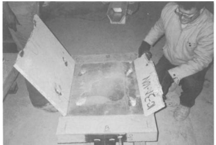
*Commentary:* Individual anchor tests evaluate the interactive capacity of the actual device with the stone it engages. It isolates the anchor and stone adjacent to it by limiting the panel size used in the test so that the failure surely occurs at the anchorage, not by stone panel breakage.
