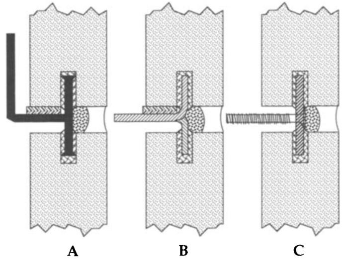
▲ **FIGURE 64: Anchor Types Than Fit Into Kerfs.** Devices that engage a kerf sawn in the stone include an extruded profile (A), a brake-formed shape (B), and a plate, or disc with a fastener tie-back (C). They may be continuous (except C) or intermittent, and typically located in the top and bottom edges due to needs for access and alignment during installation.
