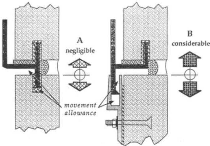
▲ FIGURE 29: *Acceptance Of Exterior Wall Dynamics Within Stone Anchorages.*
