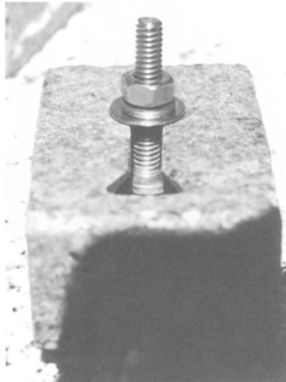
oblong head of the shank slides into the slot. The type #31 provides positive mechanical anchorage without strict dependence upon double-drilled hole alignment, torque, and rigidity of the supporting structure maintaining the shank’s stability.
