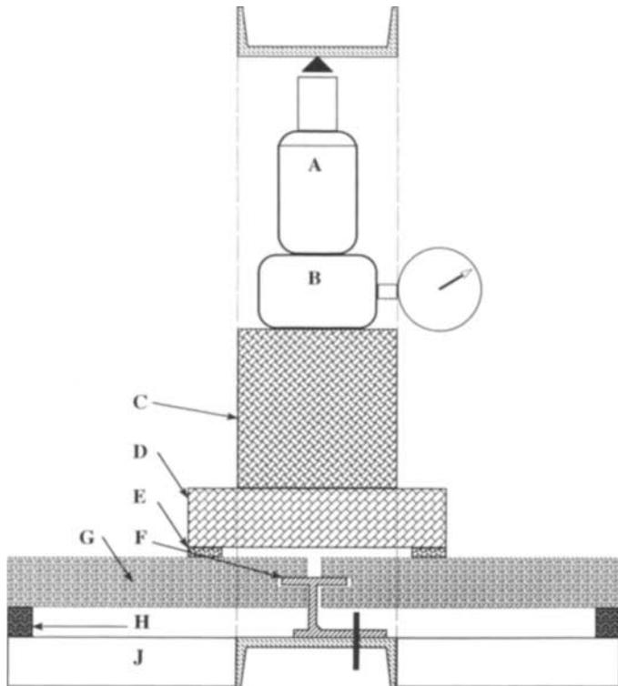
Stone Kerf Anchorage Capacity Test
