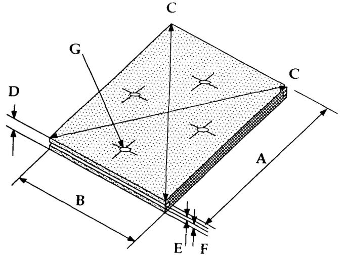
▲ FIGURE 26: *Individual Stone Fabrication Tolerances.* Practical minimum tolerances which should be expected on most normally-produced dimension stone. While many fabricators may boast better, design engineering and expectations should accommodate these variances at a minimum. As panels increase in size and thickness, these tolerances may not be sufficient:
