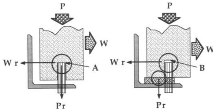
◀ FIGURE 53: *Separate Lateral and Vertical Reaction Points of Contact At The Pin.* Avoid unpredictable capacities due to complex stress flows in the stone which result from an improper single point of contact. Point contact (at A) on the pin head causes stress concentrations that cause premature breakage. A deeper hole (at B) provides clearance which prevents point contact.
