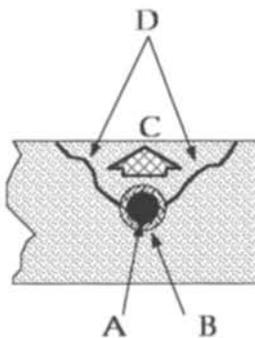
◀ FIGURE 100: *Distribution of Dowel Contact Within The Drilled Hole.* The compressible fill in the drilled hole (B) helps distribute the forces (C) transferred from the stone to the dowel in the anchor (A) bearing upon the side of the hole. Shear-tension stresses develop along a diagonal plane emanating from the line of bearing contact (D). This surface area is relatively small, developing through the height of the hole and through the edge distance in the lone of the support reaction.
