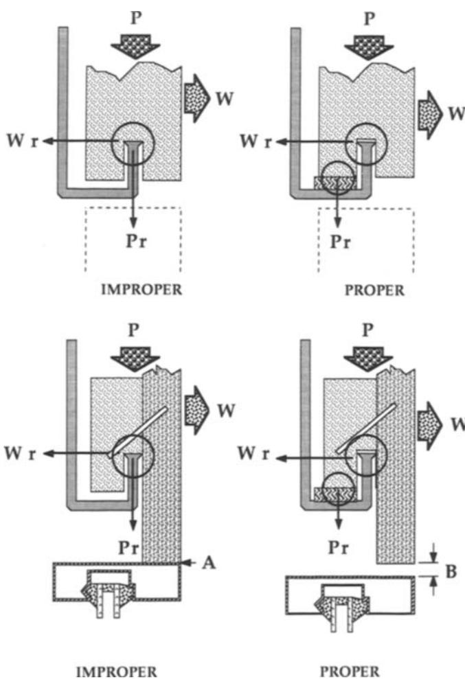
◀ FIGURE 51: *Separate Lateral and Vertical Reaction Points of Contact in the Kerf.* Complicated and unpredictable behavior results from improper support of the stones weight (P) and lateral wind load (W) at a single point of contact where gravity support (Pr) and lateral support (Wr) occur. Predictable, verifiable behavior results where gravity support (Pr) rests on the "ledge angle" independent of lateral support (Wr).
