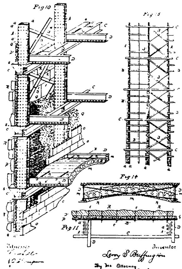
▲ FIGURE 7: *Iron Building Construction Patent (1888)*. Patented by Leroy Buffington in mid-1888, diagrams clearly show the riveted frame utilizing cross-bracing and rods for internal stability independent of the envelope. Columns use haunches at each floor as “ledges” to support that floor’s masonry exterior wall, thus relieving its weight at each floor. Drawing from *Art Bulletin* 26, March 1944.
