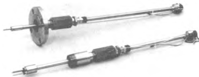
FIG. 4—Two (top) and three (bottom) electrode polarization probes for exposure in plant environments (photograph courtesy of Metal Samples Co., Inc., Munford, AL).
