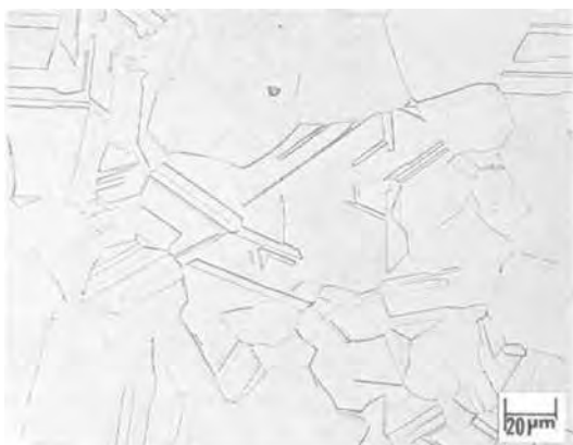
a. UNS R31233 Wrought Plate (Annealed)
