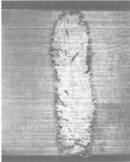
FIG. 21—Intergranular attack on weldment in ferritic stainless steel caused by high nitrogen content (5 \times ). Autogenous weld in 28.5 %Cr-4.2 %Mo alloy with 22 ppm carbon and 388 ppm nitrogen after exposure in ferric sulfate-50 % sulfuric acid test.
