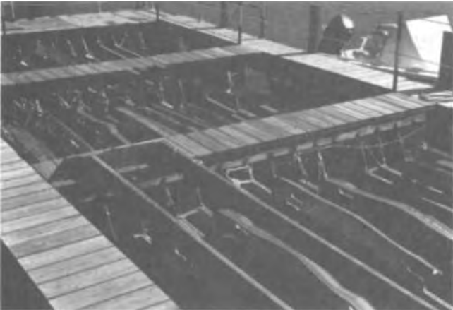
FIG. 7—Marine splash and spray exposure test on vehicle bumpers.
