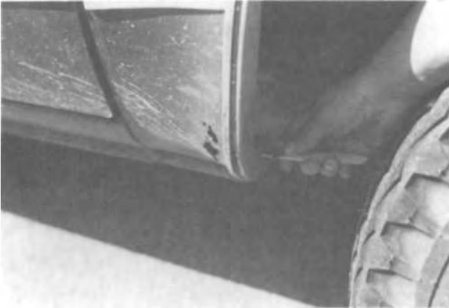
FIG. 2—Structural corrosion (inside-out perforation) on automobile body.
