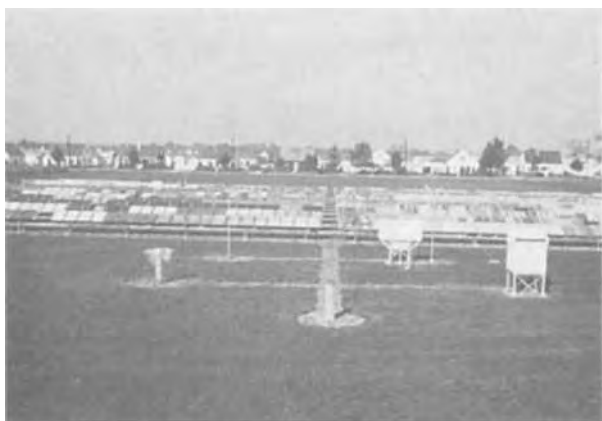
FIG. 1—Typical atmospheric corrosion test yard at Middletown, Ohio, showing exposure racks and instrumentation. Reprinted with permission of Armco, Inc. [sic]
