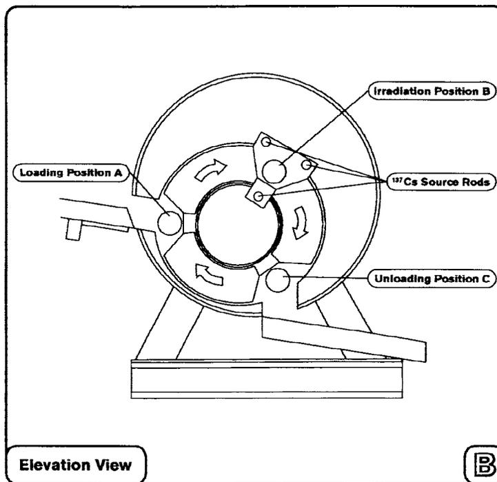
FIG. A1.2 Basic construction of the Husman <sup>137</sup>Cs irradiator
