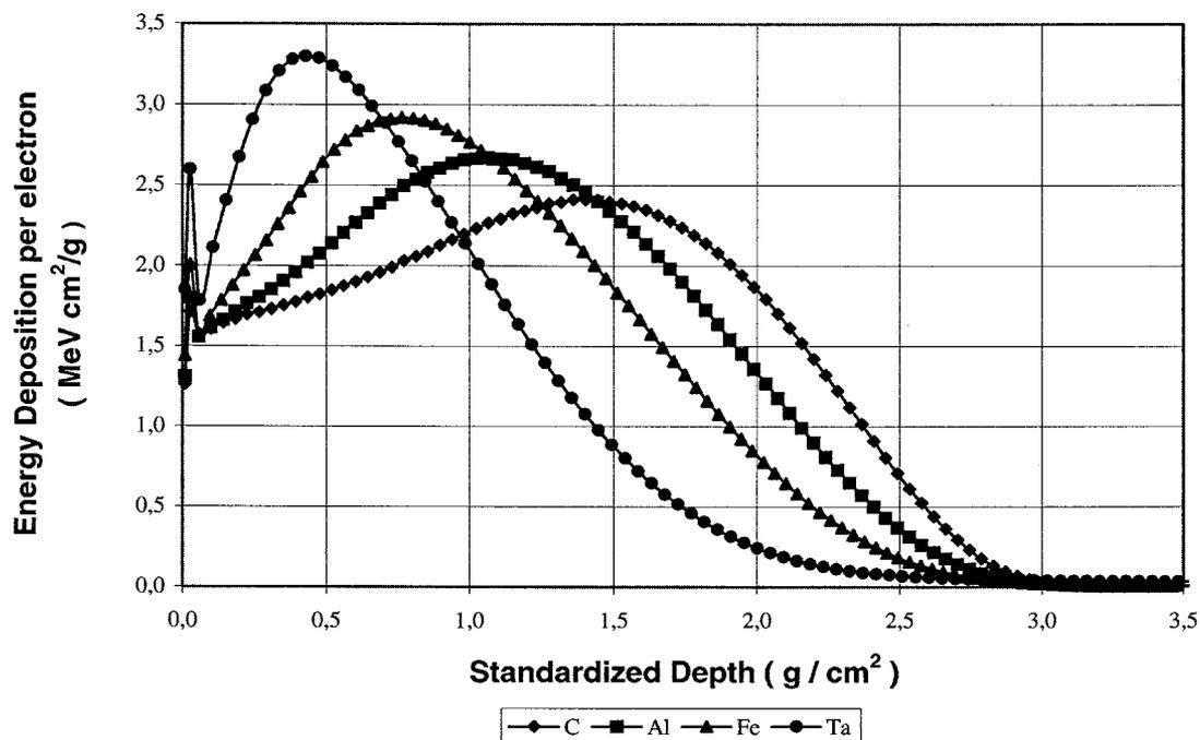
NOTE 1—The window is assumed to be  $4 \times 10^{-5}$  m thick titanium ( $0.018 \text{ g/cm}^2$ ) followed by 0.15 m of air ( $0.018 \text{ g/cm}^2$ ). The first Monte Carlo calculated data point of these curves represents the energy deposition in the titanium window and the second set of data points represents the energy deposition in the air space. The third data points correspond to the energy deposition at the surface of the irradiated material.
