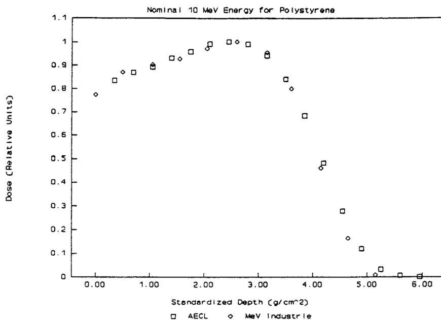
□ Example of a depth-dose distribution using a 10 MeV IMPELA linear accelerator.
