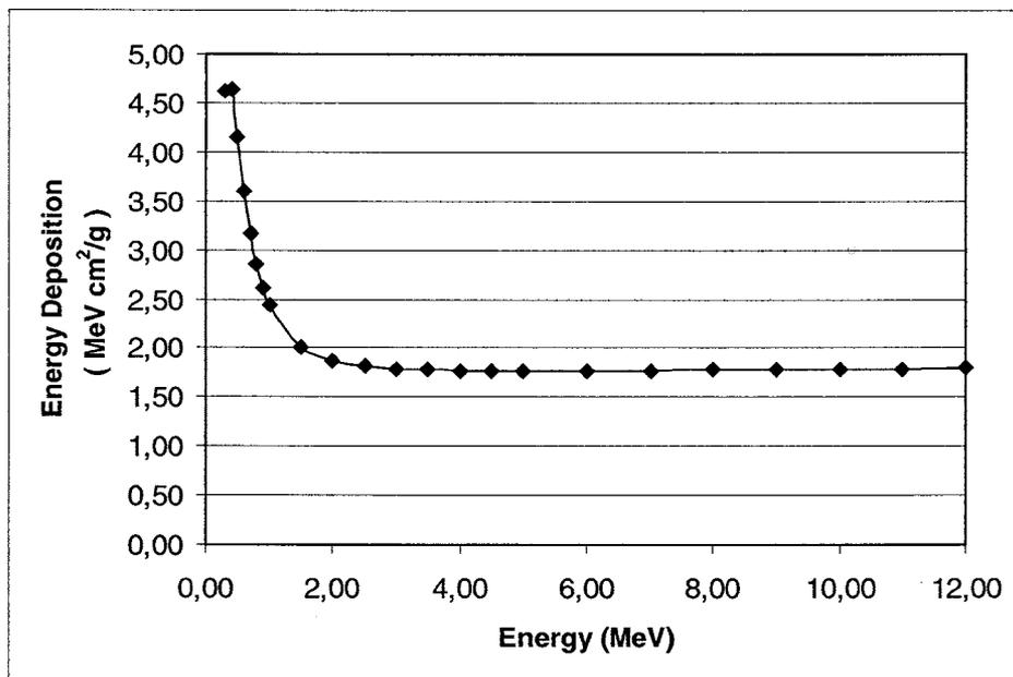
NOTE 1—The beam window is assumed to be 4 × 10<sup>-5</sup> m titanium (0.018 g/cm<sup>2</sup>) followed by 0.15 m of air (0.018 g/cm<sup>2</sup>).
