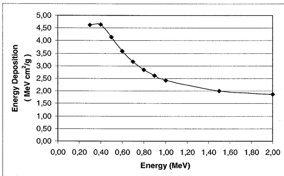
NOTE 1—The beam window is assumed to be  $4 \times 10^{-5}$  m titanium ( $0.018 \text{ g/cm}^2$ ) followed by 0.15 m of air ( $0.018 \text{ g/cm}^2$ ).
