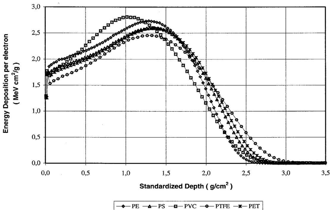
NOTE 1—The window is assumed to be  $4 \times 10^{-5}$  m thick titanium ( $0.018 \text{ g}/\text{cm}^2$ ) followed by 0.15 m of air ( $0.018 \text{ g}/\text{cm}^2$ ). The first Monte Carlo calculated data point of each curve represents the energy deposition in the titanium window and the second data point of each curve represents the energy deposition in the air space. The third data points correspond to the energy deposition at the surface of the irradiated material.
