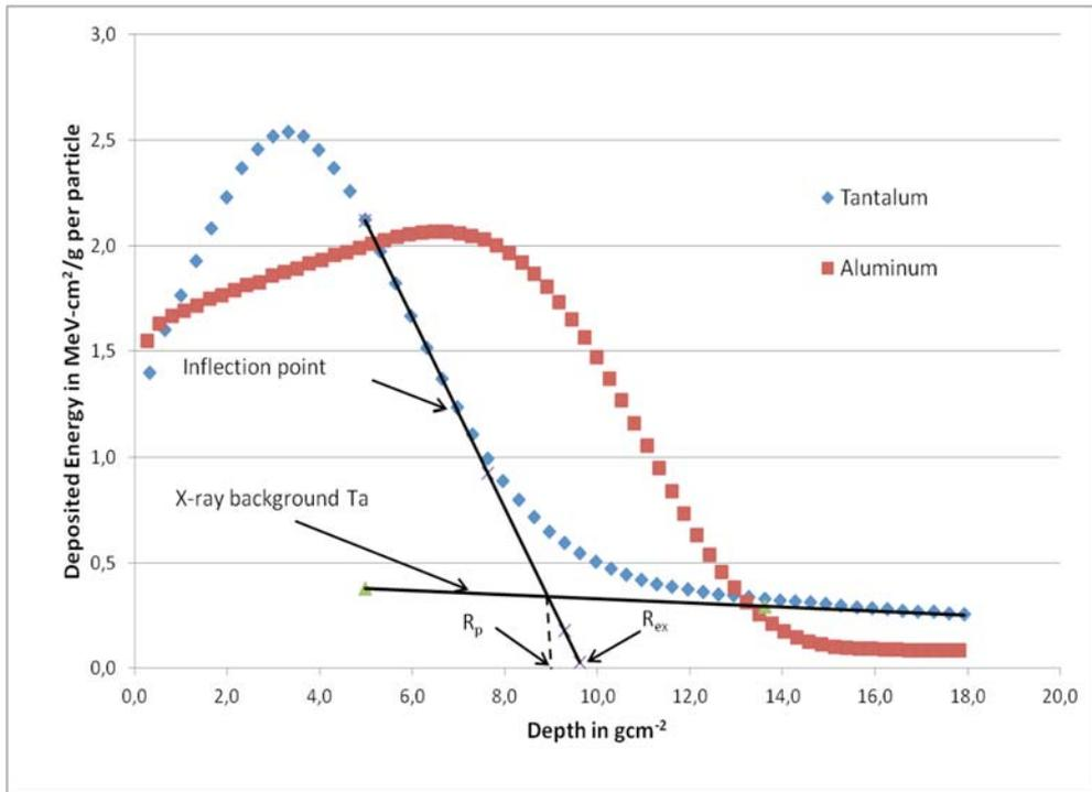
NOTE 1—The X-ray background and the definitions of electron range  $R_{ex}$  and  $R_p$  using the tangent through the inflection point are illustrated.
