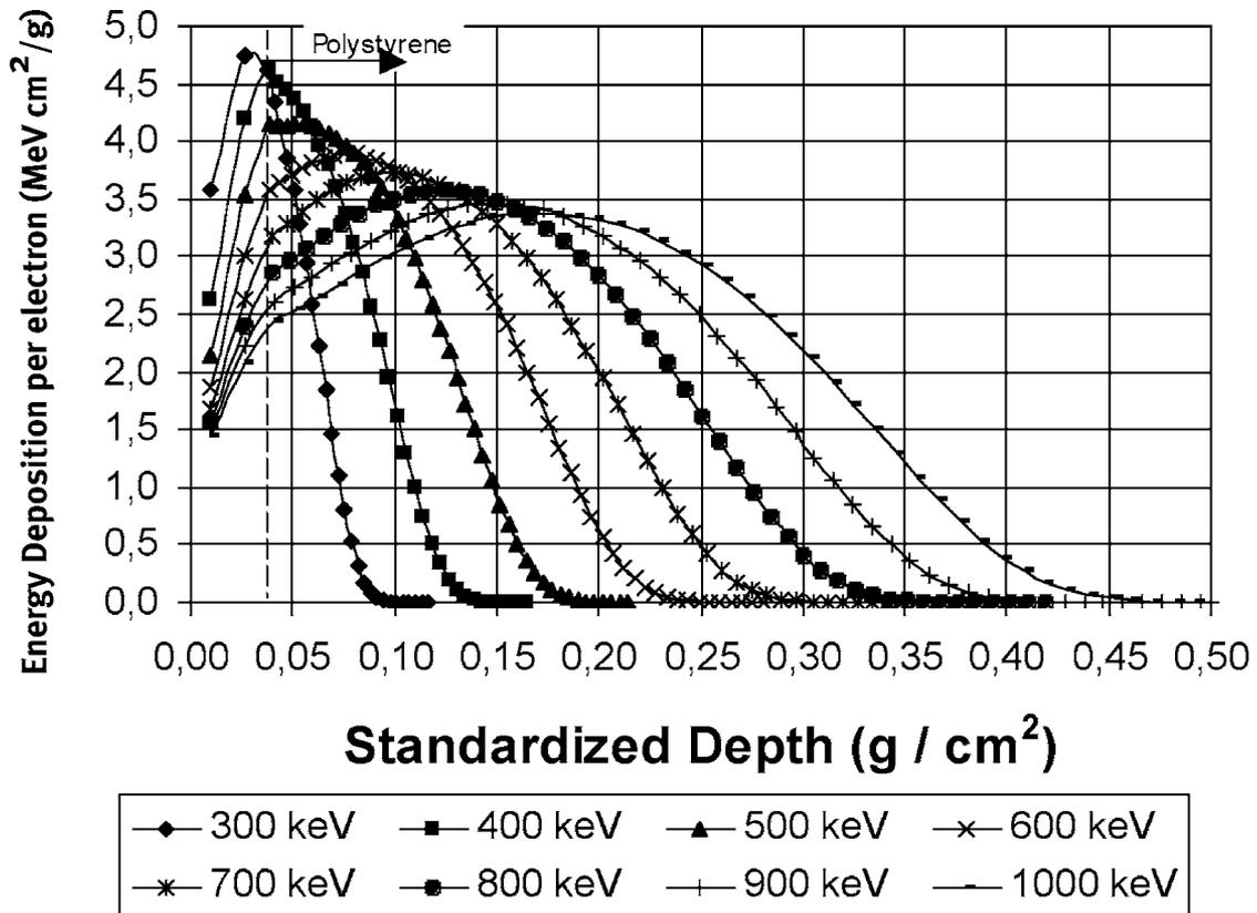
NOTE 1—The window is assumed to be  $4 \times 10^{-5}$  m thick titanium ( $0.018 \text{ g/cm}^2$ ) followed by 0.15 m of air ( $0.018 \text{ g/cm}^2$ ). The first Monte Carlo calculated data point of these curves represents the energy deposition in the titanium window and the second set of data points represents the energy deposition in the air space. The third data points correspond to the energy deposition at the surface of the irradiated material.
