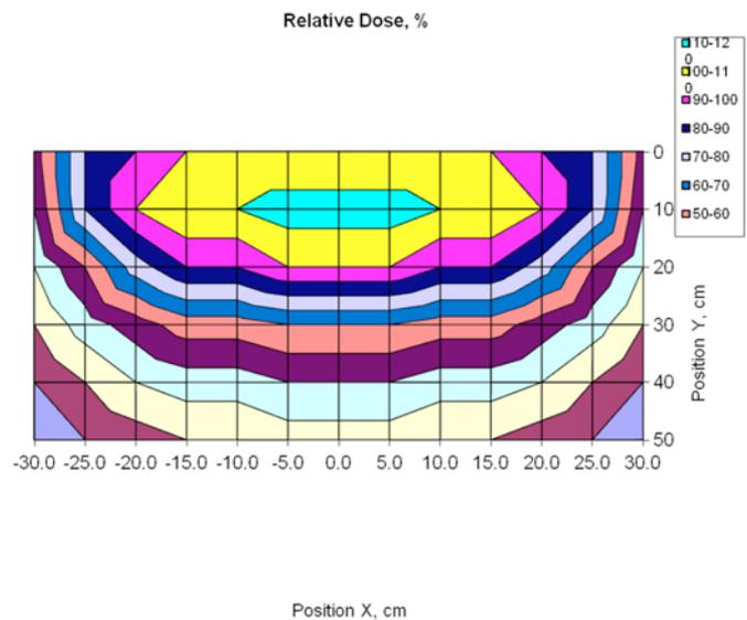
FIG. A8.1 Example of isodose curves obtained by irradiation at a 10-MeV electron accelerator of expanded polystyrene foam (specific density approximately  $0.1 \text{ g/cm}^3$ )
