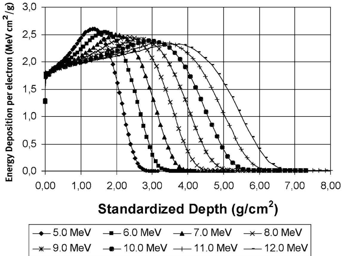
NOTE 1—The window is assumed to be  $4 \times 10^{-5}$  m thick titanium ( $0.018 \text{ g/cm}^2$ ) followed by 0.15 m of air ( $0.018 \text{ g/cm}^2$ ). The first data point of these curves represents the energy deposition in the titanium window and the second set of data points represents the energy deposition in the air space. The third data points correspond to the energy deposition at the surface of the irradiated material.
