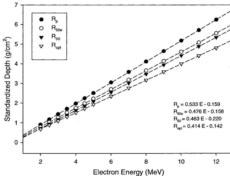
FIG. A2.9 Calculated correlations between incident electron beam energy and optimum thickness  $R_{opt}$ , half-value depth  $R_{50}$ , half-entrance depth  $R_{50e}$ , and practical range  $R_p$  for polystyrene using data from Figs. A2.4 and A2.5 (see Table A4.1)
