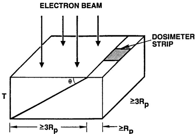
NOTE 1—Height  $T \geq 1.5 R_p$ , where  $R_p$  is the anticipated practical range of the electron beam in the wedge material (for example, aluminum).  $\theta$  is no larger than  $30^\circ$ . A film dosimeter strip is placed along the sloping surface between the two wedges.
