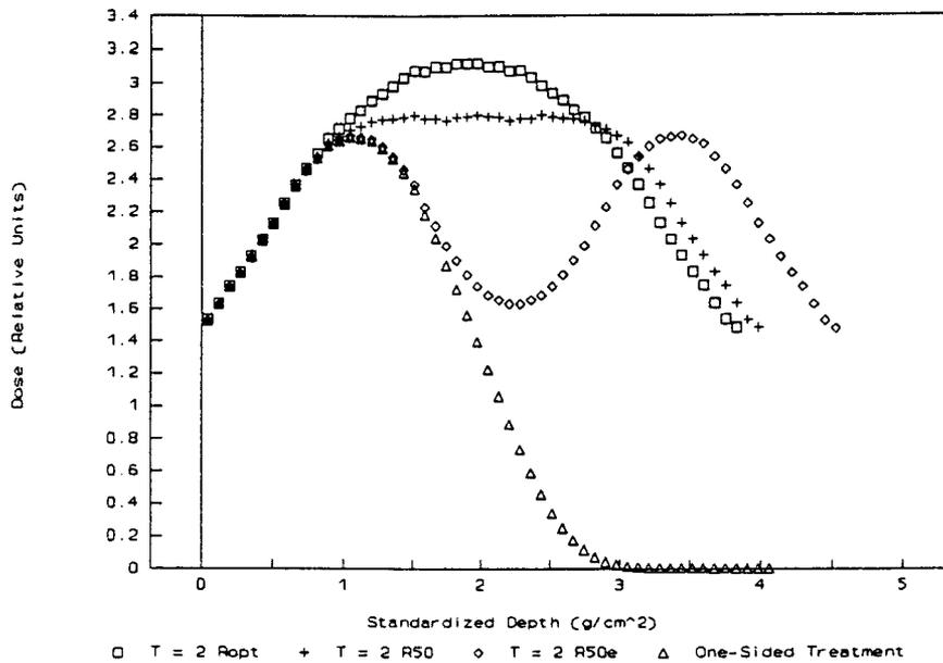
**FIG. A2.7** Superposition of calculated depth-dose distributions for aluminum irradiated with 5-MeV monoenergetic electrons from both sides with different thicknesses ( $T$ ) and from one side using experimental data presented in Refs (18 and 25) (see Notes A2.2-A2.4)
