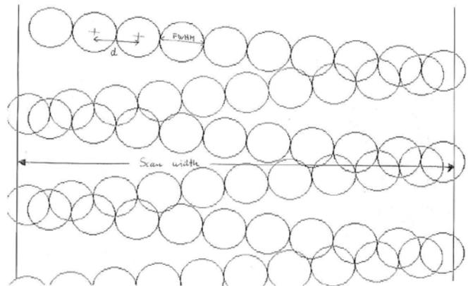
Speed, mpm: 50 Width, m: .4 Scan/sec: 20 PPS: 200 Spot Dia, mm: 40
