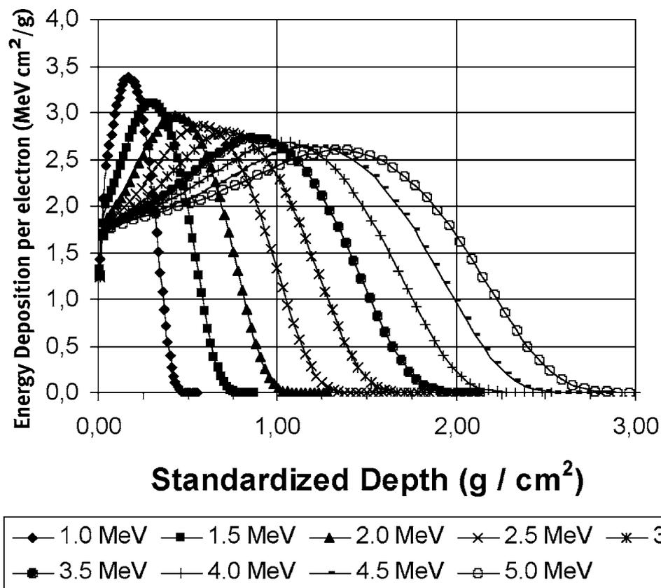
NOTE 1—The window is assumed to be  $4 \times 10^{-5}$  m thick titanium ( $0.018 \text{ g/cm}^2$ ) followed by 0.15 m of air ( $0.018 \text{ g/cm}^2$ ). The first Monte Carlo calculated data point of these curves represents the energy deposition in the titanium window and the second set of data points represents the energy deposition in the air space. The third data points correspond to the energy deposition at the surface of the irradiated material.
