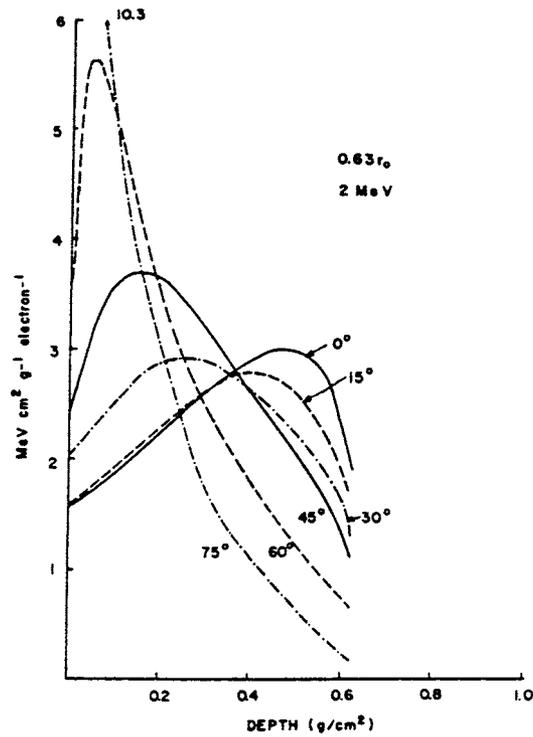
FIG. A2.12 Depth-dose distributions with 2 MeV electrons incident on polystyrene absorbers at various angles from the normal direction (31)
