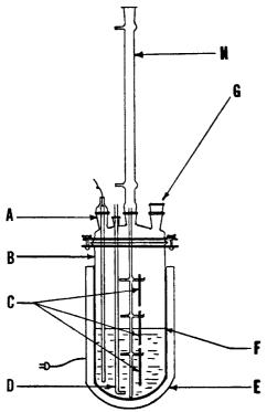
Note 1—A = thermometer port, B = flask, C = specimens hung on supporting device, D = air inlet, E = heating mantle, F = liquid interface, G = opening in flask for additional apparatus that may be required, and H = reflux condenser.
