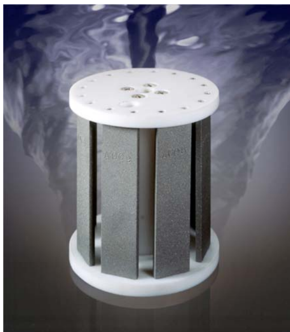
FIG. 2 Photo of Rotating Cage Containing Coupons
