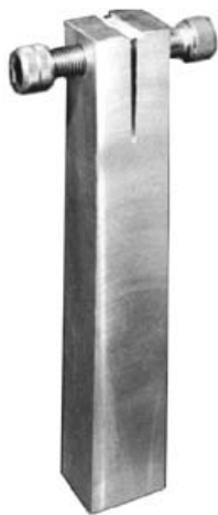
FIG. 4 Bolt Loaded Precracked Double Beam Specimen
