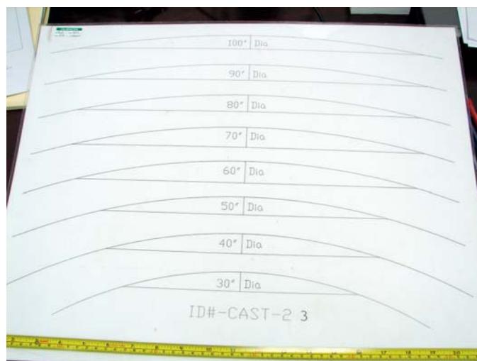
FIG. 3 Example of a Template Used for Measuring Large Diameter Spooled Wire Cast
