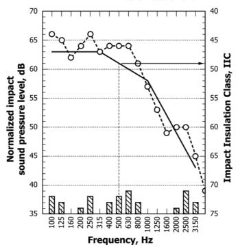
Note 1—Normalized impact sound pressure levels from a Test Method E492 measurement with an IIC rating of 49. The positive differences are shown as bars at the bottom of the plot; their sum is 27. The solid line is fitted contour. The dotted line with symbols shows the measurements.
