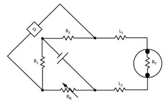
FIG. X2.1 Two-Wire Thermometer Connected to a Simple Bridge
