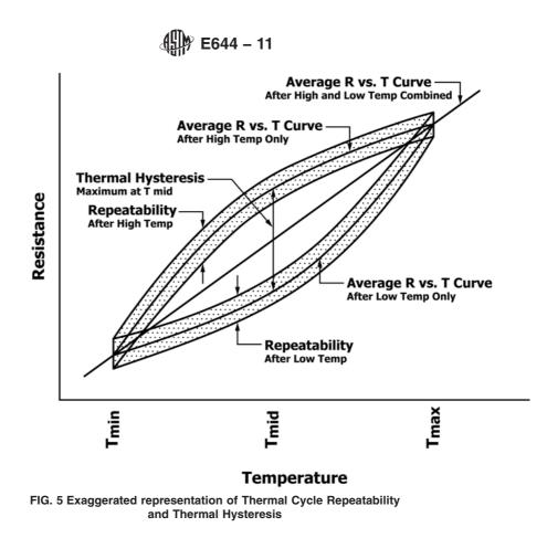
the test medium shall be within  $\pm 0.01$  °C or 25% of the thermal cycle repeatability specification, whichever is greater.
