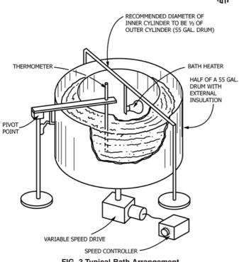
FIG. 3 Typical Bath Arrangement
