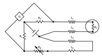
FIG. X2.3 Determination of the Resistance of a Compensated Four-Wire Thermometer Employing a Modified Bridge
