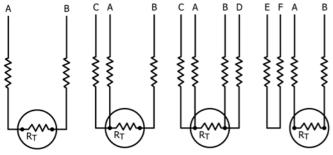
FIG. X1.1 Thermometer Wire Configurations
