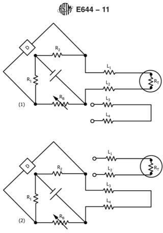
FIG. X1.3 Two-Measurement Method for Determining the Resistance of a Compensating Loop Four-Wire Thermometer Employing a Simple Bridge
