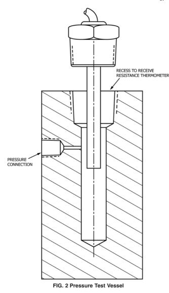
source to the vessel and attach the thermometer wires to the resistance measuring instrument. Insert the pressure vessel into the ice-point bath and allow the resistance reading to stabilize at temperature.
