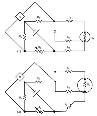
FIG. X1.2 Two Measurement Method for Determining the Resistance of a Three-Wire Thermometer Employing a Simple Bridge
