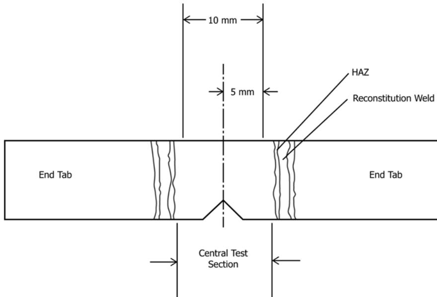
**FIG. 2 Example of Reconstituted Charpy-sized Specimen**
