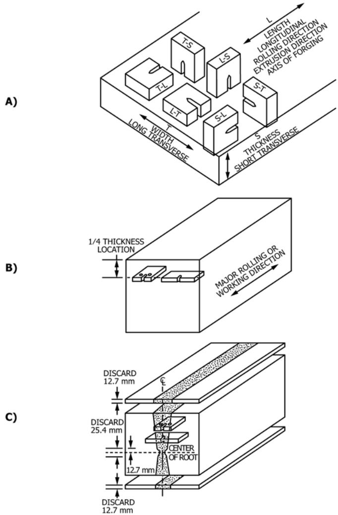
FIG. 1 Specimen Orientation and Location in Plate, Forging, and Weld Deposit Materials: A) Crack Plane Orientation Code; B) Plate and Forging Specimen Location and Orientation; C) Weld Specimen Location and Orientation
