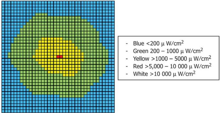
FIG. 1 Example of Beam Irradiance Profile
