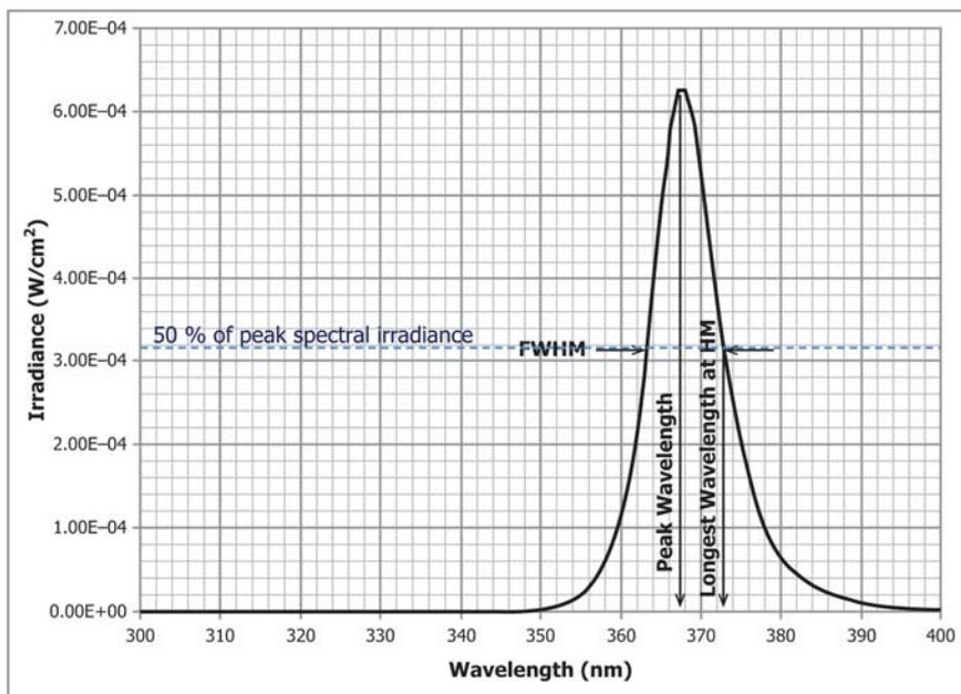
FIG. 3 Determination of Peak Wavelength, FWHM, and Longest Wavelength at Half Maximum (HM)
