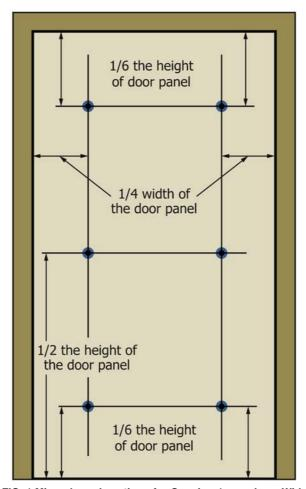
FIG. 1 Microphone Locations for Opening 1 m or Less Wide
